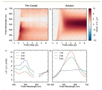
Fig. 4 Transient absorption spectra of a) a SNO thin crystal using the photoreversion approach and b) 20 mM SNO solution in hexane using only pump (0.46 mJ cm<sup>-2</sup>) and probe beams and flowing the sample. The plots were not corrected for probe dispersion. c) and d) Traces along the wavelength for different probe delays for thin crystal and solution, respectively. The region between 575 and 625 nm in the thin crystal is affected by fluctuations in the power of the NOPA beam and is masked.
