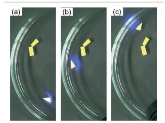
Fig. 2 (a-c) Snapshots of the motion (every 2 seconds) of the filter paper containing MeOAZ on the water surface triggered with UV light irradiation (ca. 100 mW cm<sup>-2</sup>).
