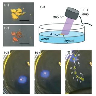
**Fig. 1** Photographs of the crystalline powders of MeOAZ on a slide glass (a) before and (b) after UV light irradiation (100 mW cm<sup>-2</sup>, 5 min). The scale bars are 5 mm. (c) Schematic diagram of the experiment of crystal motion on a water surface. (d-f) Snapshots of the crystal motion on a water surface. Line in (f) shows the trajectory of the motion. Cross marks represent the position of the crystal at every second. Numbers denote the displacement (mm) from the original position.
