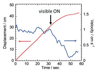
**Fig. 4** Displacement and velocity of the filter paper containing MeOAZ irradiated with visible light (450 nm, *ca.* 50 mW cm<sup>-2</sup>). The boat was previously irradiated with UV light before placing on the water surface. Velocity was determined based on the displacement every second.
