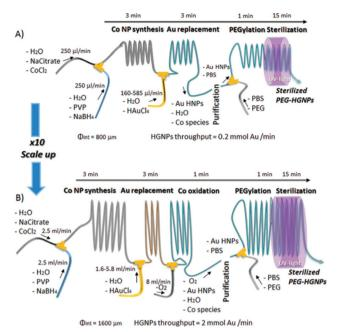
Fig. 2 Experimental set up for the production of HGNPs produced from galvanic replacement of sacrificial Co templates, including stages PEG functionalisation and sterilisation on a singular platform, scaled up for high throughput. Reprinted with permission from L. Gomez, V. Sebastian, S. Irusta, A. Ibarra, M. Arruebo and J. Santamaria, Lab Chip, 2014, 14, 325-332. Copyright (2014) Lab Chip.
