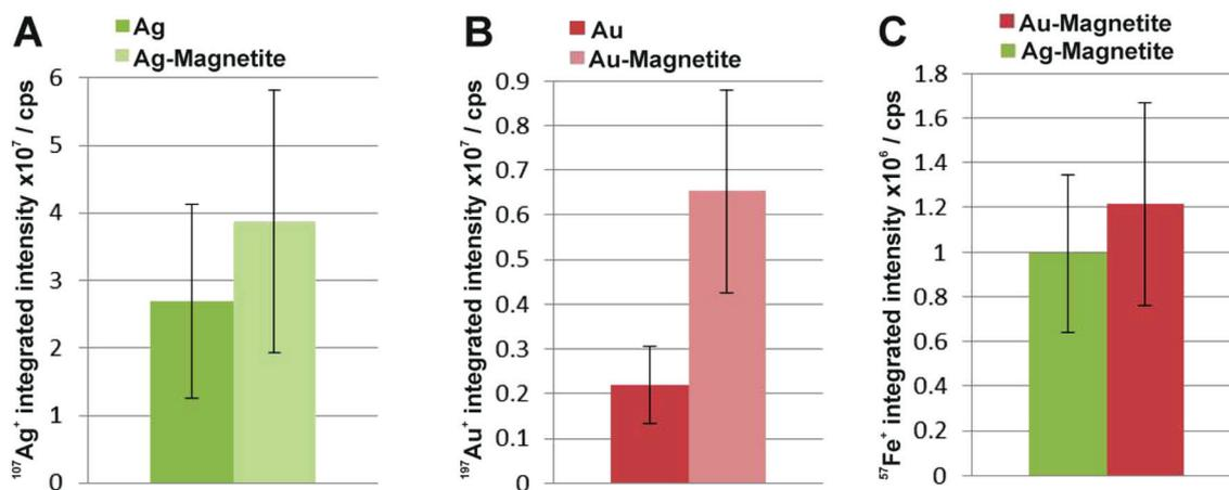
**Fig. 6** Integrated intensities of  $^{107}\text{Ag}^+$  (A),  $^{197}\text{Au}^+$  (B) and  $^{57}\text{Fe}^+$  (C) of single cells exposed to Ag–Magnetite and Au–Magnetite as well as non-linked silver and gold nanoparticles based on LA-ICP-MS data. The integrated intensities are given as the mean value of 10–20 fibroblast cells. The standard deviation reveals the cell-to-cell variability.
