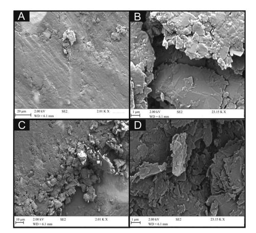
Fig. 5 SEM images of 6B PDEs drawn one (A and B) and ten times (C and D).
