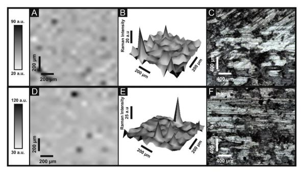
Fig. 6 2D (A and D) and 3D (B and E) schematic Raman maps generated from analysis of 6B PDEs drawn one (A, B and C) and ten (D, E and F) times respectively and their corresponding optical images (C and F). Raman intensities were recorded at the characteristic 2D peak occurring ca. 2750 cm<sup>-1</sup>.
