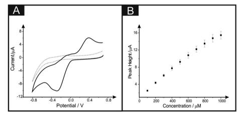
Fig. 7 Typical cyclic voltammograms (A) recorded in the absence (dotted line) and presence of 500  $\mu$ M p-benzoquinone (solid line) within a pH 7.4 phosphate buffer solution. Typical calibration plot (B) corresponding to additions of p-benzoquinone over the range of 100 to 1000  $\mu$ M into a pH 7.4 phosphate buffer solution. Recorded using a 6B PDE drawn ten times. Error bars indicate the average response and standard deviation (N = 3). Scan rate: 50 mV s<sup>-1</sup> (vs. SCE).
