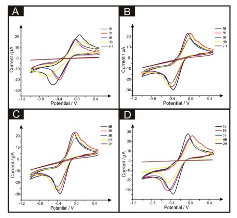
Fig. 2 Typical cyclic voltammograms utilising different pencil grades drawn one (A), three (B), five (C) and ten (D) times, recorded in 1 mM hexaammineruthenium(III) chloride/0.1 M KCl. Scan rate: 50 mV s<sup>-1</sup> (vs. SCE).
