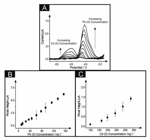
Fig. 8 Simultaneous determination of Pb( $_{\parallel}$ ) and Cd( $_{\parallel}$ ) recorded in 0.1 M HCl (dotted line) utilising a back-to-back 6B PDE drawn ten times. Shown in (A) are the corresponding linear sweep voltammograms with corresponding calibration plots (B) and (C) respectively. Error bars indicate the standard deviation of N=3. Deposition potential and time: -1.2 V (vs. SCE) and 120 seconds respectively.
