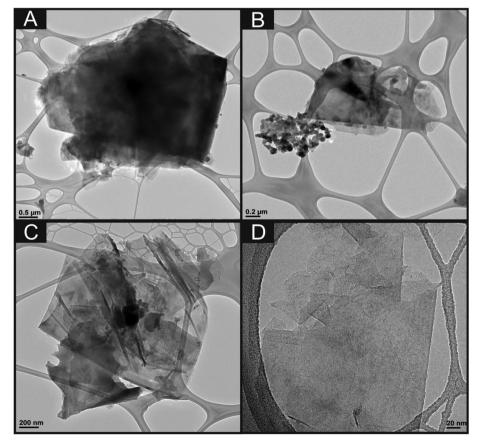
Fig. 4 TEM images of the bulk 6B pencil 'lead' (used for the fabrication of the PDEs) at increasing magnifications.
