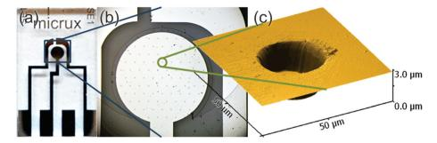
Fig. 1 (a) Photo of the thin-film microarray electrode, (b) optical microscope image of the platinum working electrode, consisting of a platinum disk electrode ( $\mathcal{O}_{\text{Pt-disk}} = 1 \text{ mm}$ ) covered by a (3.0  $\pm$  0.5  $\mu$ m thick) SU-8 layer and defined by 90 microholes ( $\mathcal{O}_{\text{u-hole}} = 10 \mu$ m, pitch = 100  $\mu$ m), (c) atomic force microscopy (AFM) mapping of a working electrode microhole.
