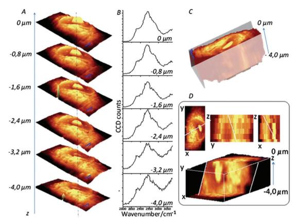
Fig. 7 Confocal Raman imaging-stack of an EA.hy 926 cell covering  $16.7 \times 34.1 \times 4 \, \mu m^3$ . Integration map (A) over the  $\nu_{C-H}$  band (2800–3020 cm<sup>-1</sup> range), single spectra (B) extracted from the same point in the maps (dotted line), a reconstructed 3D image seen from the top (C) and a cross-section of the reconstructed 3D image (D). Reproduced with permission from the Royal Society of Chemistry, Copyright 2013, ref. 99.
