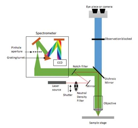
Fig. 2 Standard configuration of a confocal Raman microscope
