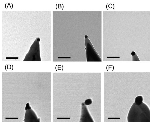
**Fig. 2** Representative TEM images of TES tips with Au@Ag NPs with various sizes (scale bar: 100 nm, see ESI, Fig. S4† for the measurement of the diameter of NP). (A)  $24 \pm 0.5$  nm, (B)  $28 \pm 0.3$  nm, (C)  $34 \pm 0.7$  nm, (D)  $50 \pm 0.4$  nm, (E)  $55 \pm 0.7$  nm, (F)  $60 \pm 0.5$  nm.
