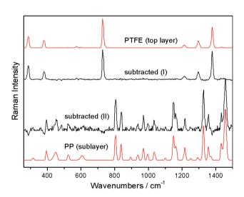
Fig. 3 Numerical recovery of pure Raman spectra of individual layers from the micro-SORS measurements carried out on the two-layer polymeric system depicted in Fig. 2: (I) recovered top layer spectrum and (II) recovered sublayer spectrum. Reference spectra are shown in top and bottom positions.17
