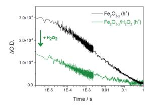
Fig. 5 TA decay traces recorded at 700 nm of photoholes on  $\alpha$ -Fe<sub>2</sub>O<sub>3-x</sub> at 1.4 V<sub>RHE</sub> in 1 M NaOH in the absence and presence of a hole scavenger (0.5 M H<sub>2</sub>O<sub>2</sub>).
