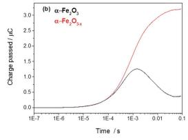
Fig. 4 (a) TPC decays of  $\alpha$ -Fe<sub>2</sub>O<sub>3</sub> and  $\alpha$ -Fe<sub>2</sub>O<sub>3-x</sub> held at 1.4 V<sub>RHE</sub> with an inset showing the overlay of the decay of the TA with the integrated TPC in Fe<sub>2</sub>O<sub>3</sub> at 1.4 V<sub>RHE</sub> (Fig. S6†) and (b) the converted total charge passed following UV excitation (355 nm, 6 ns).
