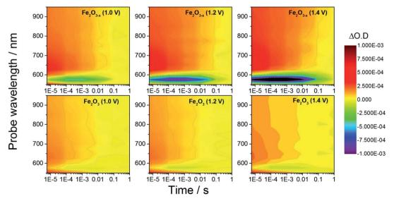
Fig. 2 TA spectra of  $\alpha$ -Fe<sub>2</sub>O<sub>3-x</sub> at various applied potentials (vs. RHE) in 1 M NaOH with the photoanodes excited from the electrolyte/electrode side (EE) with a 355 nm (6 ns pulse) laser.
