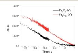
Fig. 3 TA decay traces at 700 nm of photoholes on  $\alpha$ -Fe<sub>2</sub>O<sub>3</sub> and  $\alpha$ -Fe<sub>2</sub>O<sub>3-x</sub> at 1.4 V<sub>RHE</sub> in 1 M NaOH following UV excitation (355 nm).
