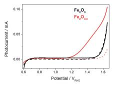
Fig. 1 Linear sweep voltammograms for  $\alpha$ -Fe<sub>2</sub>O<sub>3</sub> (black) and  $\alpha$ -Fe<sub>2</sub>O<sub>3-x</sub> (red), 5 mV s<sup>-1</sup>, under low power white light illumination (solid line, *ca.* 0.1 sun) and in the dark (dashed line).
