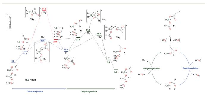
Scheme 2 Computed pathways in acetonitrile (at the M06-2X/6-311+G(d,p) level of theory) and proposed catalytic cycle for the dehydrogenation of formic acid catalyzed by BBN-H derivatives.
