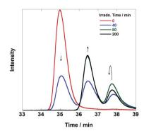
Fig. 10 Size exclusion chromatograms of the solutions before and after the photocatalytic reaction using  $Ru(CH_2SCH_2)Re$  (irradiation times: 0, 40, 80, and 200 min). The reaction and analytical conditions were the same as those described in Fig. 6.
