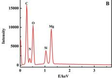
Fig. 2 SEM image (A) and EDX analysis (B) of the nanoporous MgO.
