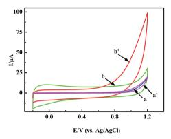
Fig. 3 CVs of the GCE (a and a'), and nanoporous MgO/GCE (b and b') in PBS solution in the absence (a and b) and presence (a' and b') of 1 mM  $\rm H_2O_2$ .
