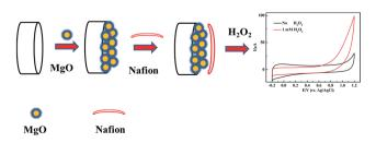
Fig. 1 Schematic diagram of the electrochemical H<sub>2</sub>O<sub>2</sub> sensor.
