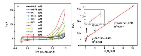
Fig. 4 (A) CV curves of the nanoporous MgO modified electrode in PBS with different concentrations of  $H_2O_2$ ; the scan rate is 50 mV s<sup>-1</sup>. (B) Sensor response curve between the magnitude of the anodic current and the  $H_2O_2$  concentration in a range from 0.05 to 0.2 mM and 0.2 to 10 mM. The inset is the linear relationship between the magnitude of the anodic current and the  $H_2O_2$  concentration in a range from 0.05 to 0.2 mM. The potential is 0.9 V.
