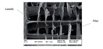
Fig. 4 SEM image of cuttlebone.
