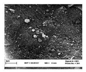
SEM image of finely powdered cuttlebone.
