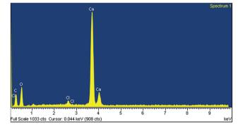
Fig. 6 EDS of finely powdered cuttlebone.
