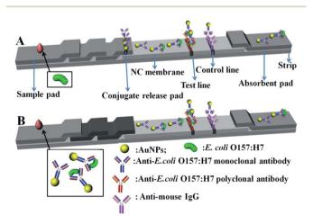
Fig. 1 Schematic of conventional (A) and modified (B) AuNP-based lateral flow immunoassay strips.
