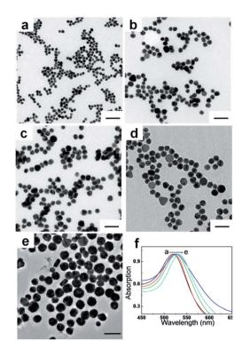
Fig. 2 Representative TEM images of AuNPs with different sizes (a): 20 nm; (b): 28 nm; (c): 35 nm; (d): 43 nm; (e): 54 nm) and their corresponding UV-Vis absorption spectra (f). The scale bar represents 100 nm.
