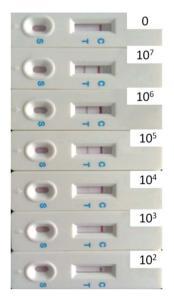
Fig. 3 Specificity of strip for the detection of *E. coli* O157:H7 (from 0 to  $10^7$  CFU mL $^{-1}$ ) using 35 nm AuNPs.
