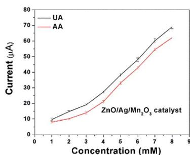
Fig. 7 Current response for different concentrations of UA and AA (1 mM to 8 mM) in the presence of ternary ZnO/Ag/Mn<sub>2</sub>O<sub>3</sub> nanocomposite modified GCE.
