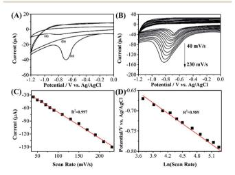
Fig. 3 (A) CVs of bare (a) GCE, (b and c) RGO–Au/GCE in 0.1 M PBS (pH 7.0) with and without 10  $\mu$ M phoxim. Scan rate: 50 mV s. (B) CVs of RGO–Au/GCE in 10  $\mu$ M phoxim at different scan rates (40, 50, 60, 70, 80, 90, 110, 130, 150, 170, 190, 210 and 230 mV s<sup>-1</sup>). (C) The plot for the dependence of peak current on the scan rate. (D) The relationship between  $E_{pa}$  and ln  $\nu$ .
