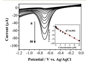
Fig. 5 DPV curves for phoxim at RGO-Au/GCE with different concentrations of phoxim (from a to m: 0.008, 0.02, 0.05, 0.1, 0.25, 0.5, 1, 2, 3, 4, 6, 8, 10 µM).
