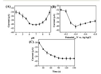
Fig. 4 Effect of the (A) pH of PBS, (B) accumulation potential and (C) accumulation time on the current response of 10 µM phoxim at RGO-Au/GCE.
