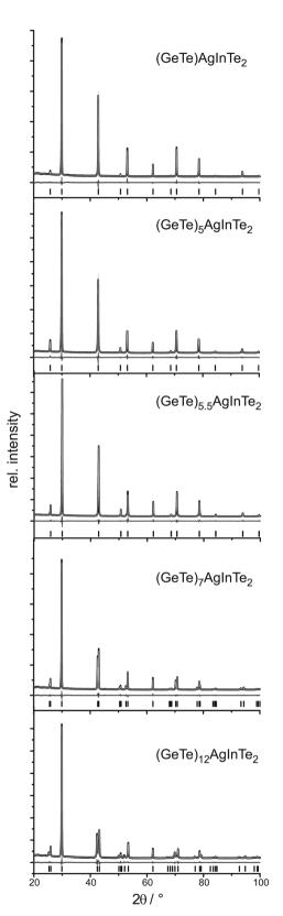
Fig. 1 Rietveld fits for  $(GeTe)_x$ AgInTe<sub>2</sub> (x = 1, 5, 5.5, 7 and 12; from top)to bottom – HP synthesis except for x = 12): experimental (black) and calculated data (gray); difference plot (gray, below); and peak positions (black, vertical lines).
