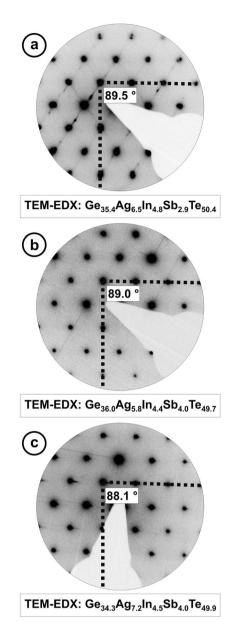
Fig. 3 SAED patterns of the  $\langle 100 \rangle$  zone axis of different crystallites in a sample of (GeTe)\_5,5AgIn\_0,5Sb\_0,5Te\_2 (a and b: different areas of the same crystallite, c: other crystallite). The [012]\* (horizontal) and [014]\* (vertical) directions are marked with dotted lines and the angle between them is given; TEM-EDX analyses of the corresponding areas are given below each SAED (calculated composition: Ge\_36,7Ag\_6,7In\_3,3Sb\_3,3Te\_50).
