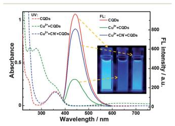
Fig. 1 UV-vis absorption and FL spectrum of 0.168 mg mL $^{-1}$  BPEICQDs (red lines), 150  $\mu M$  Cu $^{2+}$  + 0.168 mg mL $^{-1}$  BPEI-CQDs (green lines), and 2 mM CN $^{-}$  + 150  $\mu M$  Cu $^{2+}$  + 0.168 mg mL $^{-1}$  BPEI-CQDs (blue lines) in pH 7 PBS. The inset shows the corresponding photos of the three solutions illuminated by an UV beam of 365 nm.
