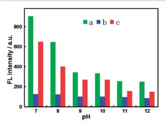
Fig. 3 FL responses of 16.8  $\mu$ g mL $^{-1}$  BPEI-CQDs (a), 15  $\mu$ M Cu $^{2+}$  + 16.8  $\mu$ g mL $^{-1}$  BPEI-CQDs (b), and 150  $\mu$ M CN $^{-}$  + 15  $\mu$ M Cu $^{2+}$  + 16.8  $\mu$ g mL $^{-1}$  BPEI-CQDs (c) at different pH values.
