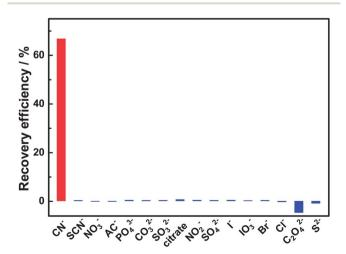
Fig. 6 Selectivity of the BPEI-CQDs/Cu $^{2+}$  system sensor for CN $^-$  over other ions in pH 7 PBS: concentrations of BPEI-CQDs and Cu $^{2+}$  were 16.8  $\mu g$  mL $^{-1}$  and 15  $\mu$ M respectively; concentrations of all anions were 150  $\mu$ M.
