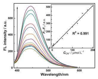
Fig. 5 FL response of BPEI-CQDs/Cu<sup>2+</sup> system (BPEI-CQDs: 16.8  $\mu$ g mL<sup>-1</sup>, Cu<sup>2+</sup> 15  $\mu$ M) upon addition of various concentrations of CN<sup>-1</sup> ions in a pH 7 PBS solution (from bottom: 0, 2, 4, 6, 8, 10, 25, 50, 75, 100, 125, 150, 175, 200  $\mu$ M). Inset: linear range of the plot of "recovered" FL intensity against the concentration of CN<sup>-1</sup> (2–200  $\mu$ M).
