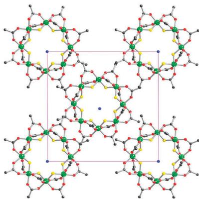
Fig. 1 Unit cell of  $\text{Cr}_7\text{Zn}@Ga_7\text{Zn}$  viewed down the crystal  $c$  axis: Ga/Cr/Zn (green), F (yellow), O (red), N (blue), C (black), Me groups omitted for clarity. See Fig. S1 (ESI $^\dagger$ ) for full molecule.
