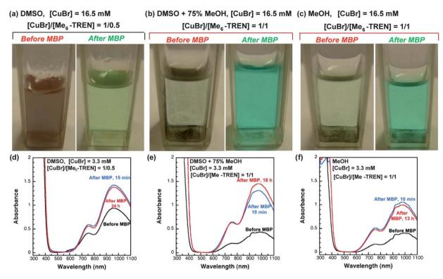
Fig. 10 Visual observation of Cu(0) nanoparticles and supporting UV-vis spectra of  $CuBr_2$  generated from the disproportionation of  $CuBr/Me_6$ -TREN in DMSO (a and d); DMSO + 75% MeOH (b and e); and MeOH (c and f) before and 10 min after the addition of MBP at 25 °C. Conditions: solvent = 1.8 mL, [MBP]/[CuBr]/[Me $_6$ -TREN] = 10/1/0.5 (a and d); [MBP]/[CuBr]/[Me $_6$ -TREN] = 10/1/1 (b, c, e and f); [CuBr] = 16.5 mM (a-c); [CuBr] = 3.3 mM (d-f).
