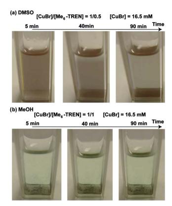
**Fig. 4** Visual observation comparing the stability of Cu(0) nanoparticles generated from the disproportionation of CuBr/Me<sub>6</sub>-TREN in DMSO (a); and MeOH (b) at 5, 40 and 90 min after mixing the reagents at 25 °C. Conditions: solvent = 1.8 mL, [CuBr] = 16.5 mM, (a) [CuBr]/[Me<sub>6</sub>-TREN] = 1/0.5 and (b) [CuBr]/[Me<sub>6</sub>-TREN] = 1/1.
