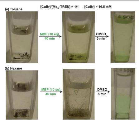
Fig. 11 Visual observation of Cu(0) nanoparticles and CuBr<sub>2</sub> generated from the disproportionation of CuBr in toluene (a); and hexane (b) before and after reaction the with MBP at 25 °C. MBP was added to the disproportionation mixtures after 40 min, followed by addition of 1.8 mL of DMSO. Conditions: solvent = 1.8 mL, [CuBr] = 16.5 mM, [MBP]/[CuBr]/[Me<sub>6</sub>-TREN] = 10/1/1.
