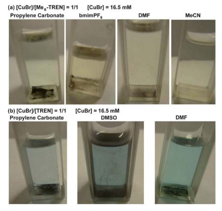
Fig. 2 Visual observation of Cu(0) nanoparticles and CuBr<sub>2</sub> generated from the disproportionation of CuBr in polar aprotic solvents in the presence of Me<sub>6</sub>-TREN (a); and TREN (b). Conditions: solvent = 1.8 mL; [CuBr]/[N-ligand] = 1/1. Pictures were taken 10 min after mixing the reagents.
