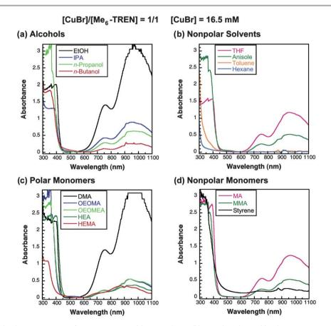
Fig. 9 UV-vis spectra of the disproportionation of CuBr/Me<sub>6</sub>-TREN in (a) protic solvents; (b) nonpolar solvents; (c) polar monomers; and (d) nonpolar monomers. Conditions: solvent or monomer = 1.8 mL, [CuBr] = 16.5 mM, [CuBr]/[Me<sub>6</sub>-TREN] = 1/1.
