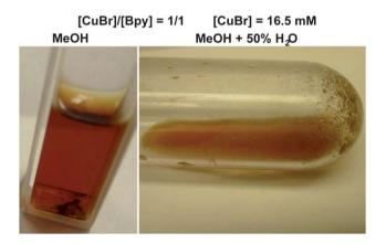
**Fig. 5** Visual observation of the disproportionation of CuBr–bpy in MeOH and MeOH + 50%  $H_2O$  at 25 °C. Conditions: solvent = 1.8 mL, [CuBr] = 16.5 mM, [CuBr]/[bpy] = 1/1. Pictures were taken 10 min after mixing the reagents.
