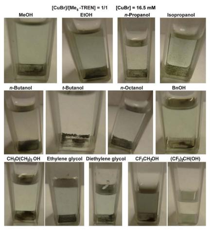
Fig. 3 Visual observation of Cu(0) nanoparticles and CuBr<sub>2</sub> generated from the disproportionation of CuBr/Me<sub>6</sub>-TREN in a range of alcohols at 25 °C. Conditions: solvent = 1.8 mL, [CuBr] = 16.5 mM, [CuBr]/[Me<sub>6</sub>-TREN] = 1/1. Pictures were taken 10 min after mixing the reagents.
