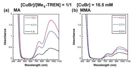
Fig. 8 UV-vis spectra of the disproportionation of CuBr/Me<sub>6</sub>-TREN in MA (a); and MMA (b) over time. Conditions: monomer = 1.8 mL, [CuBr] = 16.5 mM, [CuBr]/[Me<sub>6</sub>-TREN in MA (a); and MMA (b) over time. TREN] = 1/1.
