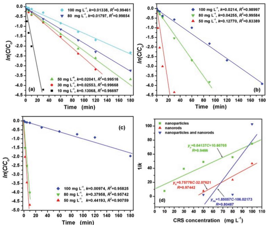
**Fig. 7** The effect of initial CRS concentration on the degradation kinetics for 50 mL CR solution at different time intervals: (a) 100 mg CeO<sub>2</sub> nanoparticles, (b) 20 mg CeO<sub>2</sub> nanorods, (c) 150 mg CeO<sub>2</sub> mixture of nanoparticles and nanorods, and (d) the relationship between the degradation rate constant  $k$  and CRS concentrations from 10 to 100 mg L<sup>-1</sup>.
