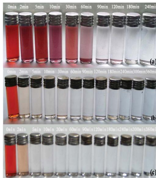
**Fig. 6** Photographs of CR solutions (CRS) before and after treatment with CeO<sub>2</sub> at different time intervals: (a) CRS (100 mg L<sup>-1</sup>, 50 mL) in the presence of 250 mg of CeO<sub>2</sub> nanoparticles, (b) CRS (50 mg L<sup>-1</sup>, 50 mL) in the presence of 20 mg of CeO<sub>2</sub> nanorods, and (c) CRS (80 mg L<sup>-1</sup>, 50 mL) in the presence of 150 mg of the CeO<sub>2</sub> mixture of nanoparticles and nanorods.
