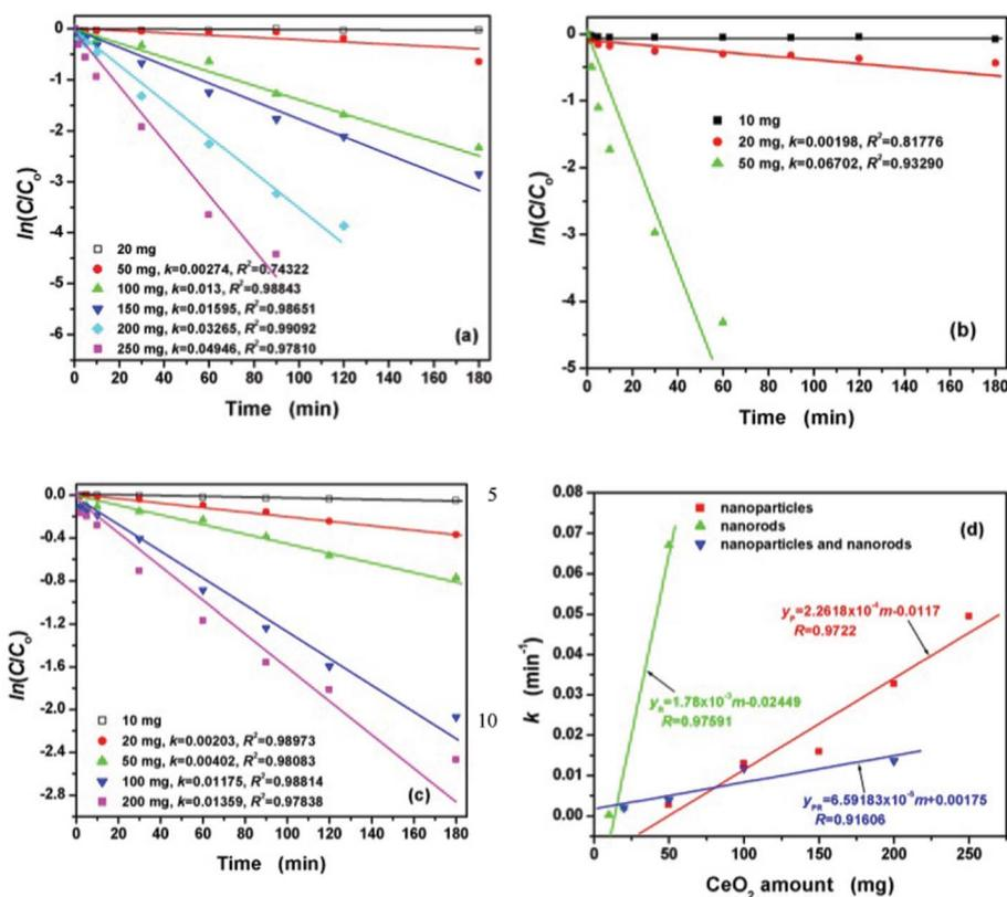
**Fig. 8** The effect of the amount of CeO<sub>2</sub> nanostructures on the degradation kinetics for 50 mL CRS (100 mg L<sup>-1</sup>) at different time intervals: (a) CeO<sub>2</sub> nanoparticles, (b) CeO<sub>2</sub> nanorods, (c) CeO<sub>2</sub> mixture of nanoparticles and nanorods, and (d) the relationship between the degradation rate constant  $k$  and the amounts of CeO<sub>2</sub> nanostructures from 10 to 250 mg.
