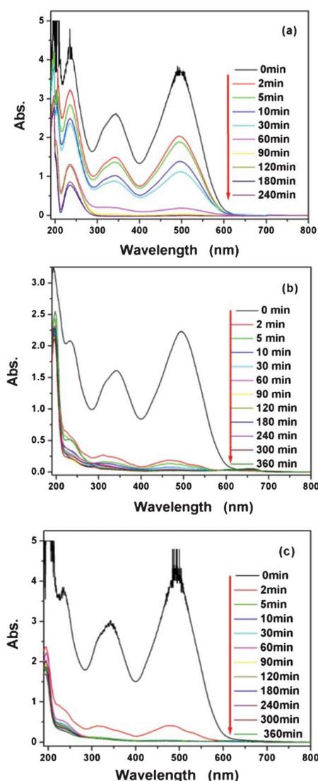
**Fig. 5** UV-Vis absorption spectra of CR solutions (CRS) before and after treatment with CeO<sub>2</sub> at different time intervals: (a) CRS (100 mg L<sup>−1</sup>, 50 mL) in the presence of 250 mg of CeO<sub>2</sub> nanoparticles, (b) CRS (50 mg L<sup>−1</sup>, 50 mL) in the presence of 20 mg of CeO<sub>2</sub> nanorods, and (c) CRS (80 mg L<sup>−1</sup>, 50 mL) in the presence of 150 mg of the CeO<sub>2</sub> mixture of nanoparticles and nanorods.
