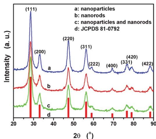
**Fig. 1** XRD patterns of as-synthesized CeO<sub>2</sub> nanostructures.
