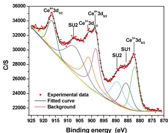
Fig. 9 XPS spectrum of CeO<sub>2</sub> nanoparticles.
