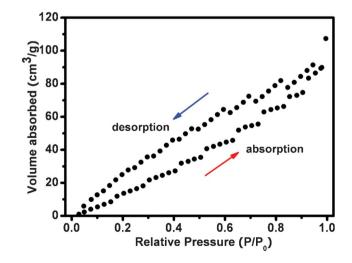
Fig. 3  $N_2$  adsorption–desorption isotherm of a 3D grapheme/ZnO hybrid.
