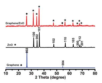
**Fig. 4** Typical XRD patterns of 3D graphene, ZnO and graphene/ZnO hybrid.
