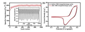
**Fig. 6** (a) The cycle performance of graphene/ZnO hybrid electrode at the current density of  $6.70 \text{ A g}^{-1}$  in 2.0 M KOH solution. The inset shows the charge–discharge profile for the graphene/ZnO hybrid electrode. (b) CV of graphene/ZnO hybrid electrode before and after 1000 charge–discharge cycles.
