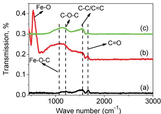
**Fig. 8** FTIR transmittance spectra of (a) GNS, (b) M1-GNS and (c) residual graphene sheets from M1-GNS after removing Fe<sub>3</sub>O<sub>4</sub> nanoparticles.
