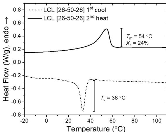
**Figure 2.** DSC of LCL triblock copolymer after precipitation with a heating/cooling rate of  $10\text{ °C min}^{-1}$ . Traces represent the first cool and second heat.
