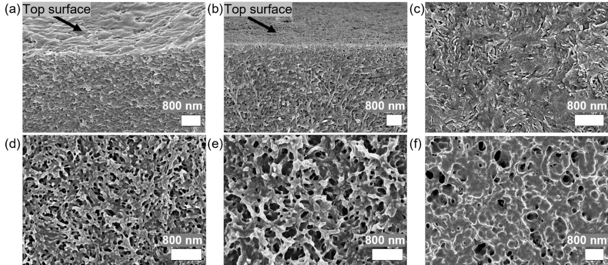
**Figure 6:** (a–b) SEM images of cryo-fractured nanoporous PCOE membranes taken near the surface of membranes derived from LCL [25-51-25]. Both samples were solvent cast followed by annealing for 20 minutes at 70 °C prior to PLA etching. Additionally, sample (b) was plasma etching for 60 seconds following PLA etching. (c–f) Surface SEM images of membranes plasma-etched for (c) 0 seconds, (d) 60 seconds, (e) 120 seconds, and (f) 600 seconds.
