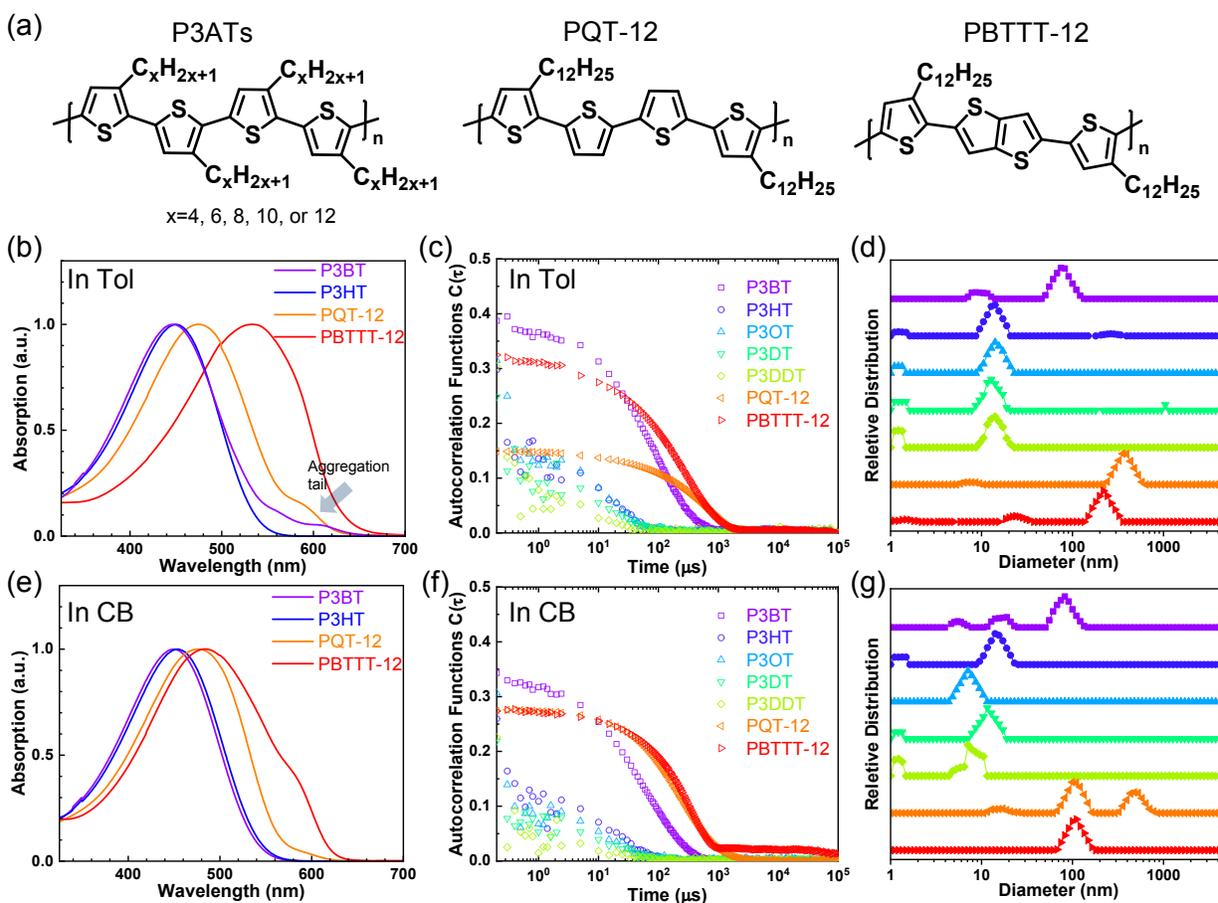
**Figure 1** (a) Chemical structure of P3ATs, PQT-12 and PBTTT-12. The UV-Vis absorption spectrum of CPs in toluene (b) and CB (e) at 20°C. Autocorrelation curve of CPs in toluene (c) and CB (f) from DLS measurement at 20°C. Size distribution of CPs in toluene (d) and CB (g) from DLS measurement.
