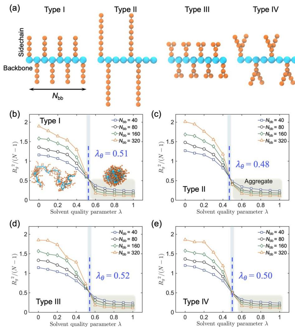
**Figure 4** CG MD simulation results. (a) Polymer architectures of 4 types of CPs. The backbone and sidechain are represented as beads P1 and P2, respectively. (b-e) Reduced  $R_g$  of polymer chain as a function of solvent quality parameter  $\lambda$  for type I to IV, respectively. A lower value of  $\lambda$
