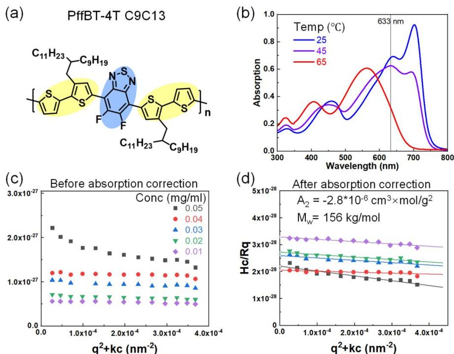
**Figure 3** (a) Chemical structure of PffBT4T-C9C13. The donor part and acceptor part are colored as yellow and blue units, respectively. (b) UV-Vis of PffBT4T-C9C13 in CB at various temperatures. The laser wavelength used in the light scattering test is marked in a gray line. (c, d) SLS of PffBT4T-C9C13 in CB at 65°C before and after absorption correction, respectively.
