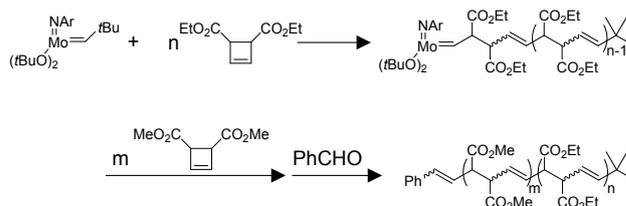
Figure 8. ROMP of 3,4-difunctionalised cyclobutenes reported by Novak et al.<sup>71</sup>
