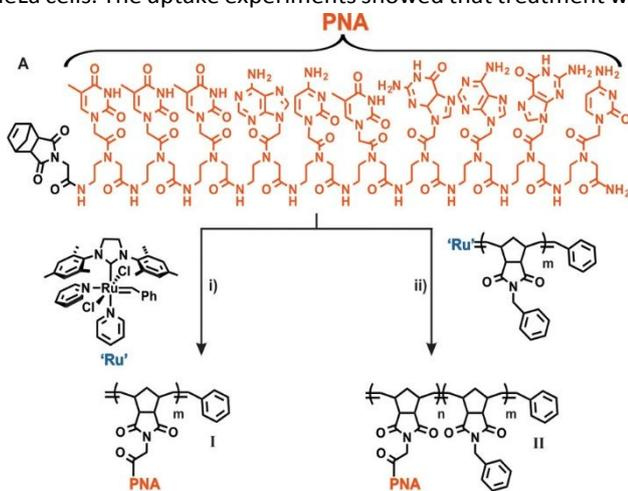
Figure 27. PNA synthesis reported by Gianneschi et al.<sup>229</sup> Figure 1A was adapted from ref. 229 with permission. Copyright 2014 American Chemical Society.
