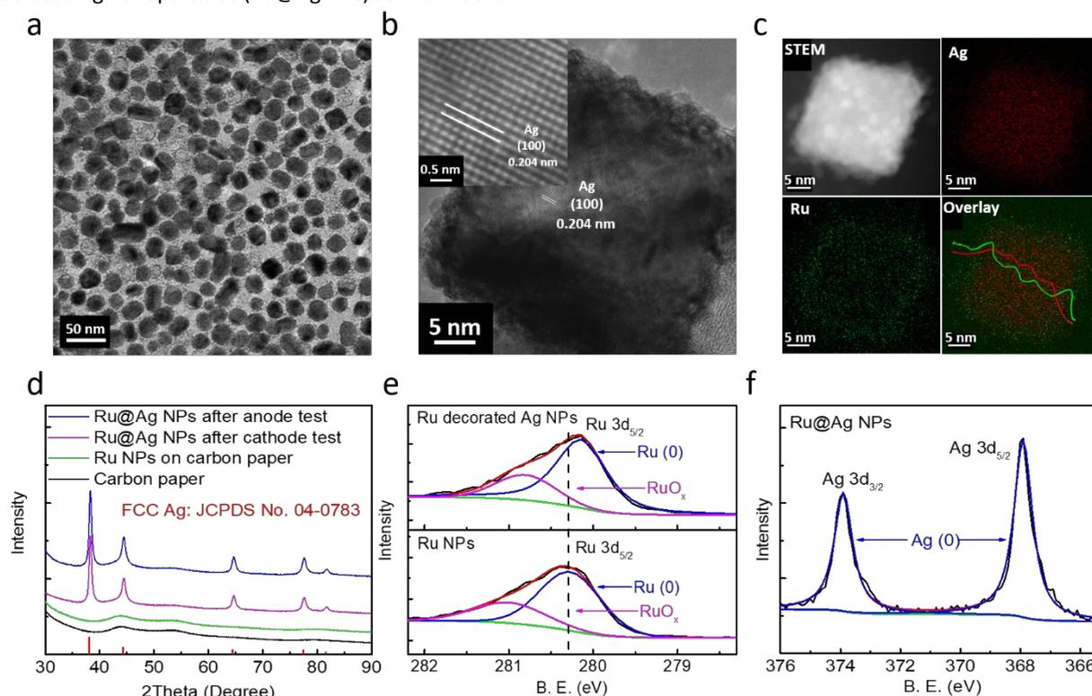
**Fig. 1** (a) TEM image of Ru@Ag NPs. (b) HRTEM image of Ru@Ag NPs. (c) STEM and EDX characterizations of Ru@Ag NPs with the line-scans for Ru (green line) and Ag (red line) shown in the lower-right panel. (d) XRD characterization of Ru@Ag NPs under working conditions, small Ru NPs and carbon paper. (e) XPS spectra of Ru for Ru@Ag NPs and small Ru NPs. (f) XPS spectra of Ag for Ru@Ag NPs.
