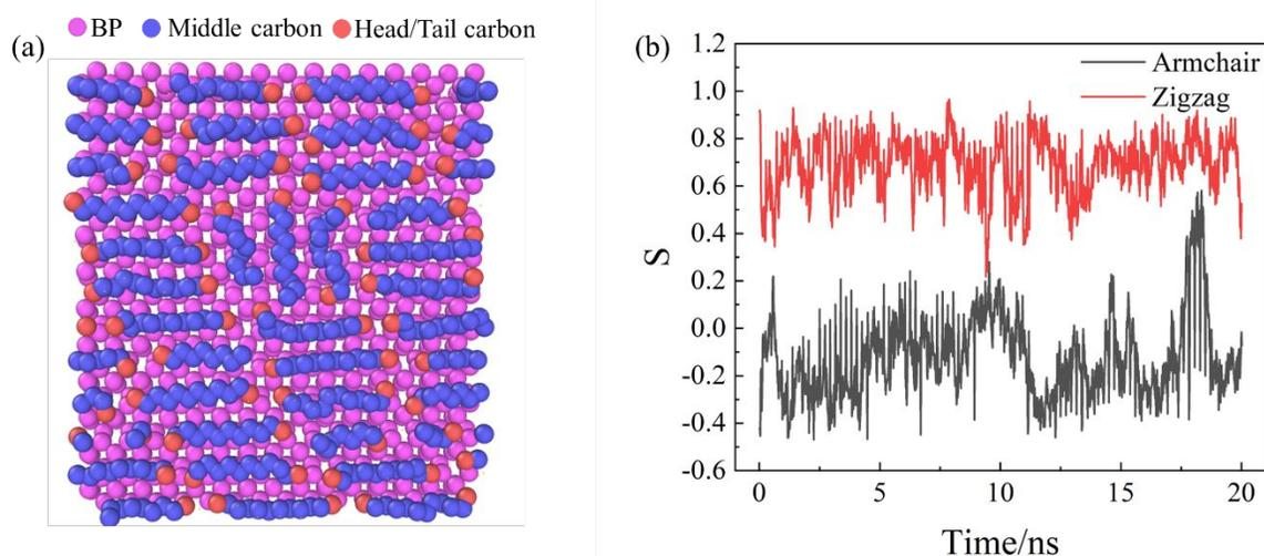
**Figure 4.** (a)  $x - z$  cross-sectional view of the one-layered structure, in which the molecular chains of  $C_{12}$  are aligned parallel to the BP wall. (b) The orientation parameter  $S$  value versus time along armchair and zigzag directions in 2-nm BP nanochannels.
