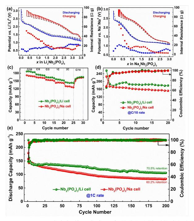
**Figure 5**. GITT curve and calculated internal resistance for (a)  $Nb_2(PO_4)_3/Li$  and (b)  $Nb_2(PO_4)_3/Na$  cells. Rate capability (c), capacity retention at C/10 (d) and 1 C (e) plots of  $Nb_2(PO_4)_3/Li$  and  $Nb_2(PO_4)_3/Na$  cells.
