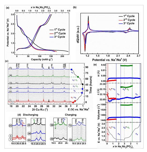
**Figure 3.** (a) Voltage vs. capacity and (b) dQ/dV profiles of Nb<sub>2</sub>(PO<sub>4</sub>)<sub>3</sub>/Na cell. (c and d) *In-situ* XRD patterns of Nb<sub>2</sub>(PO<sub>4</sub>)<sub>3</sub> anode and (e) its cell parameter evolution during the first cycle of Na-ion (de)intercalation (vertical solid and dotted lines indicate the phase boundaries during Na-ion (de)intercalation).
