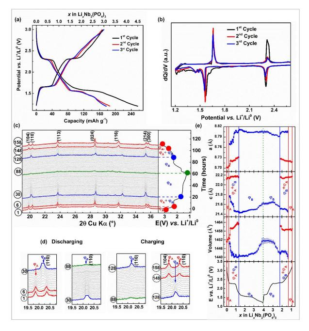
**Figure 2.** (a) Voltage vs. capacity and (b) dQ/dV profiles of Nb<sub>2</sub>(PO<sub>4</sub>)<sub>3</sub>/Li cell. (c and d) *In-situ* XRD patterns of Nb<sub>2</sub>(PO<sub>4</sub>)<sub>3</sub> anode and (e) its cell parameter evolution during the first cycle of Liion (de)intercalation (vertical solid and dotted lines indicate the phase boundaries during Li-ion (de)intercalation).
