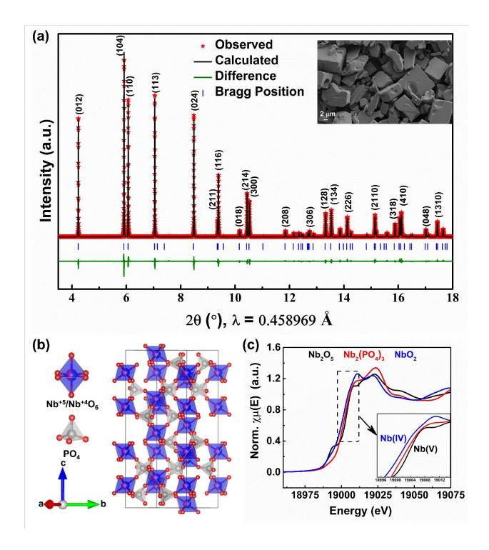
**Figure 1.** (a) Rietveld refinement of room temperature synchrotron XRD pattern (Inset: SEM image), (b) crystal structure, and (c) XANES collected at Nb K-edge of NASICON-Nb<sub>2</sub>(PO<sub>4</sub>)<sub>3</sub>.
