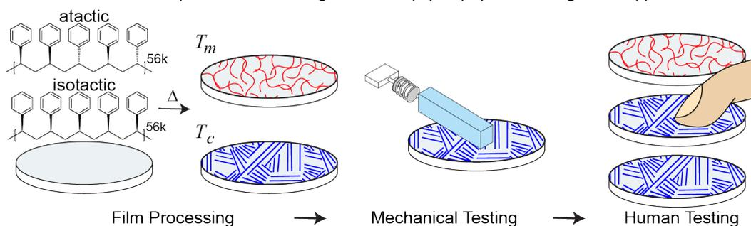
**Figure 1: Schematic of approach overview.** Polystyrene films of varying morphology are processed through differences in tacticity and isothermal annealing ( $T_m$ : Melting Temperature,  $T_c$ : Crystallization Temperature), evaluated with mechanical testing to form predictions, and then validated with human psychophysical testing.
