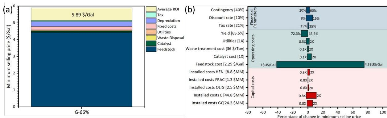
**Figure 11.** (a) Breakdown of the MFSP (b) tornado plot showing the sensitivity of the MFSP to changes in different parameters of interests (y-axis). The value within the bracket on the y-axis represents the value of the parameter in the reference case. GC: Guerbet coupling, E: etherification, OLIG: oligomerization, FRAC: fractionation, HEN: Heat Exchanger Network.
