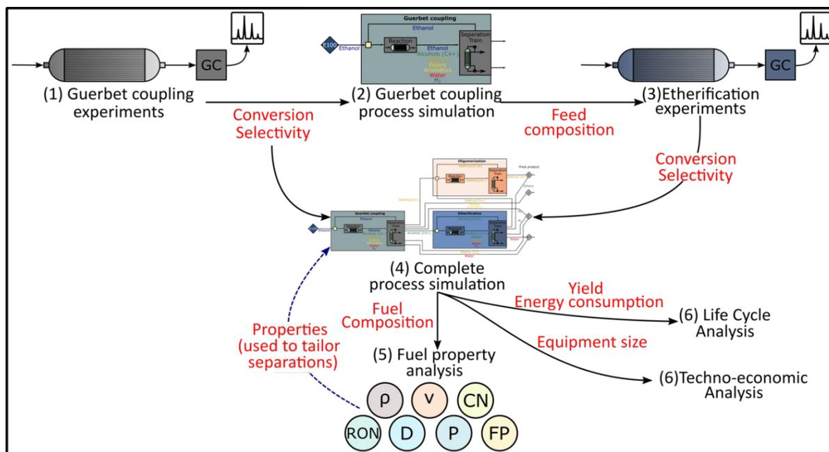
**Figure 2.** Approach followed in this work to couple experimental and simulation results. The flow of information at the different stages is shown in red fonts
