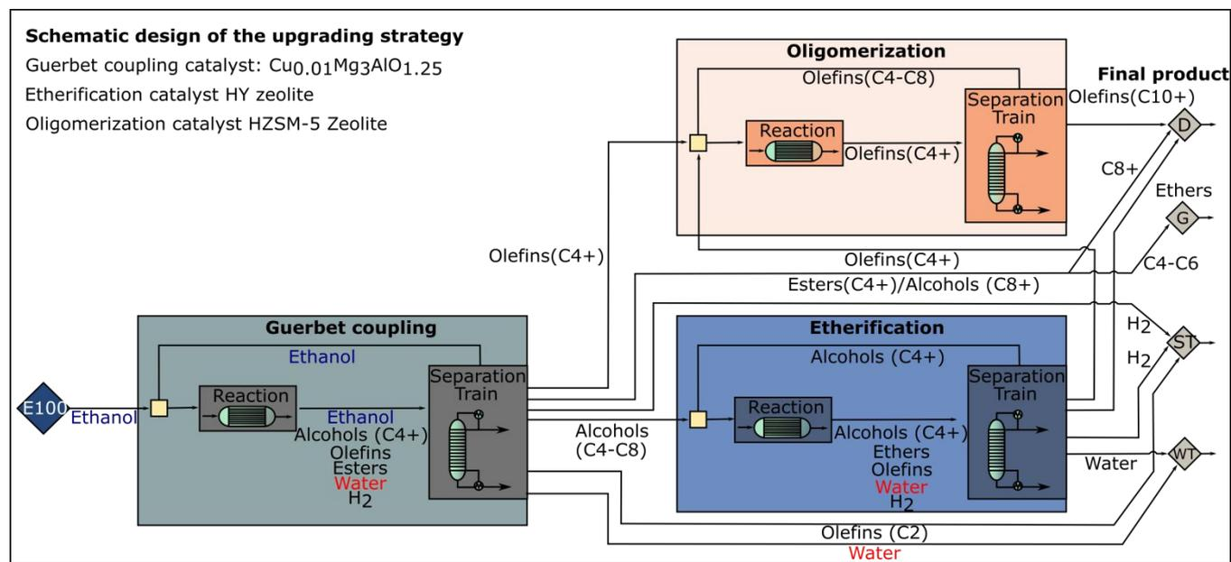
**Figure 1.** Schematic representation of an ethanol upgrading biorefinery based on Guerbet coupling, etherification, and olefin oligomerization. D: Diesel, G: Gasoline, ST: Steam, WT: Waste water.
