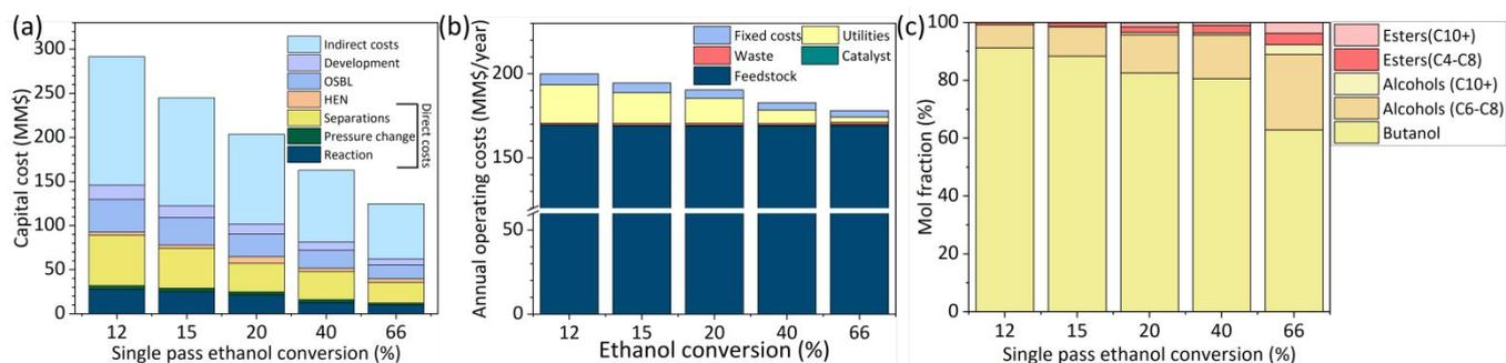
**Figure 5.** (a) Capital costs (b) annualized operating costs (c) and composition of the etherification feed stream as a function of conversion for the Guerbet coupling area. Details on the capital costs and operating conditions can be found in SI-4
