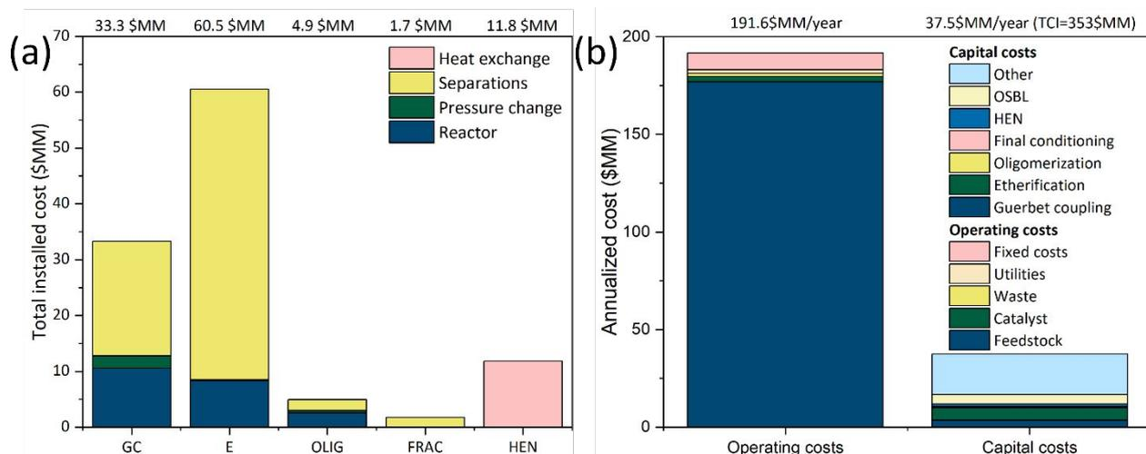
**Figure 10.** (a) Installed capital costs of the different areas in the biorefinery (b) Annualized capital and operating costs. GC: Guerbet coupling, E: etherification, OLIG: oligomerization, FRAC: fractionation, HEN: heat exchanger network, OSBL: outside battery limits.
