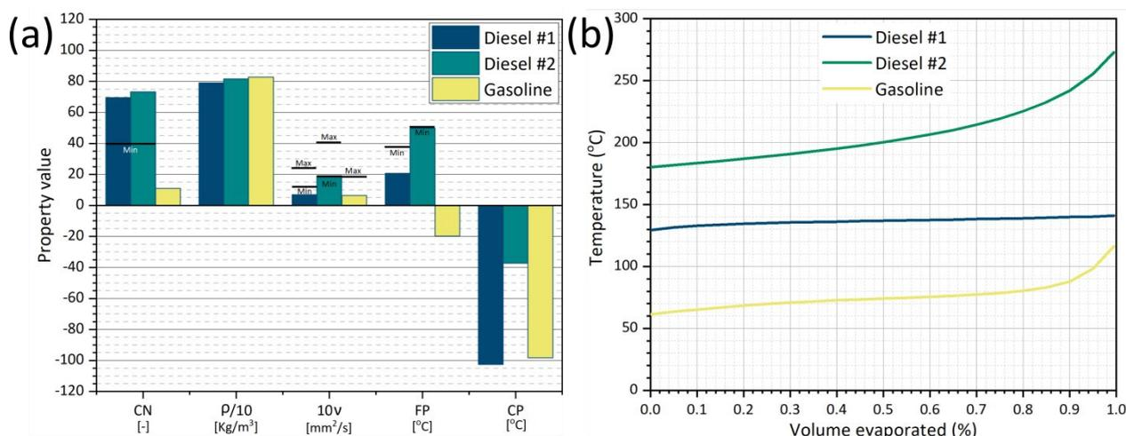
**Figure 9.** (a) Properties of the different fuels produced. CN: cetane number, D: density, V: viscosity, FP: flash point, CP: cloud point. The ASTM requirements for the properties that are constrained are indicated by horizontal black lines (b) Distillation curve of the fuels produced.
