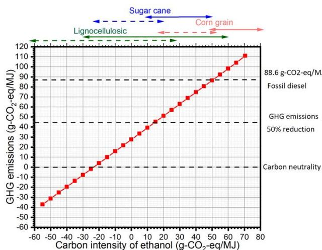
**Figure 13.** Greenhouse gas emissions as a function of ethanol carbon intensity (g-CO<sub>2</sub>-eq/MJ-Ethanol). Typical ranges for ethanol produced from lignocellulosic residues, sugar cane, and corn grain are shown on top of the figure. Dashed lines correspond to the range of carbon intensities that could be obtained if CO<sub>2</sub> capture at the fermentation outlet is implemented.
