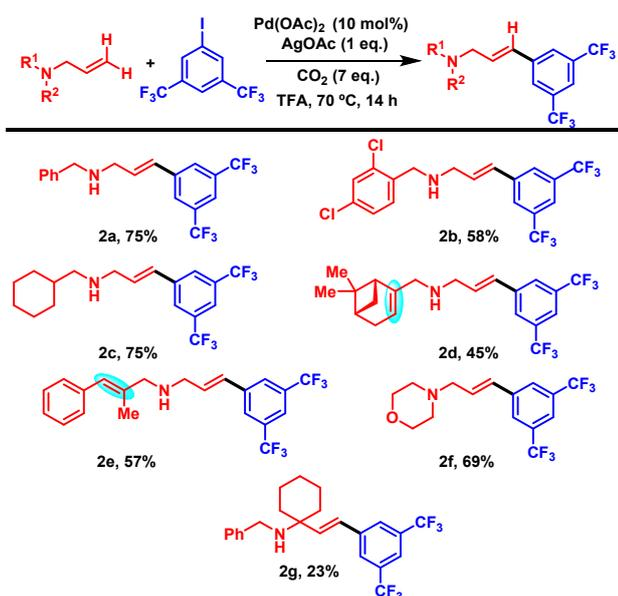
**Table 2.** Substrate Scope for Amines. Reaction conditions: allylamine (0.36 mmol), aryl iodide (0.3 mmol),  $\text{Pd}(\text{OAc})_2$  (10 mol%),  $\text{AgOAc}$  (0.3 mmol),  $\text{CO}_2$  (7 eq.) and TFA (1 mL), heated at  $70^\circ\text{C}$  for 14 h.
