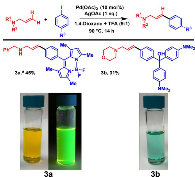
**Table 3.** Substrate Scope for Amines. Reaction conditions: allylamine (0.36 mmol), aryl iodide (0.3 mmol),  $\text{Pd}(\text{OAc})_2$  (10 mol%),  $\text{AgOAc}$  (0.3 mmol), and 9:1 dioxane and TFA (1 mL), heated at  $90^\circ\text{C}$  for 14 h. [a]  $\text{CO}_2$  (7 eq.) were added during the reaction.
