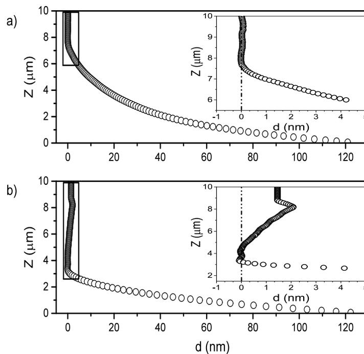
**Figure 4.** Examples of the force curves demonstrating the uncertainty in defining the effective Young's modulus and PB layer parameters when experimentally identifying zero force (zero deflection of the AFM cantilever). (a) A well-defined zero deflection. (b) An uncertain zero deflection; the insert is a zoom version of the curve highlighted by the square box.
