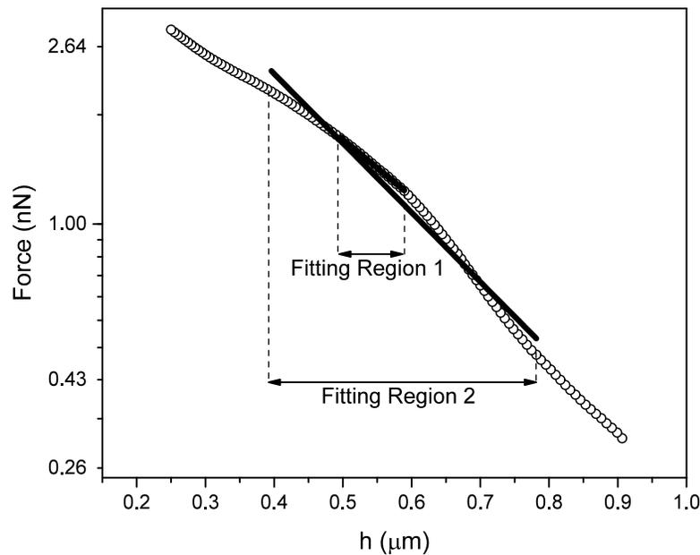
**Figure 8.** Uncertainty due to the freedom in choosing the length of the fitting region to calculate the parameters of the PB layer, the brush length, and grafting density (Step 2, optional parameterization of the PB layer). Zebrafish melanocyte cells were used for analysis.
