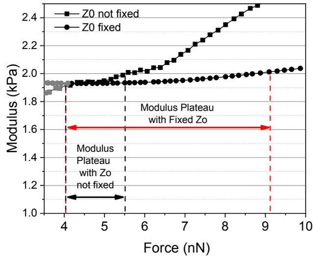
**Figure 3.** An example of dependence of the Young's modulus on the indentation depth/force. The modulus is found by fitting the experimental data using two approaches when treating  $Z_0$  is a fitting parameter and when it is fixed. The plateau is substantially increased when  $Z_0$  is fixed.
