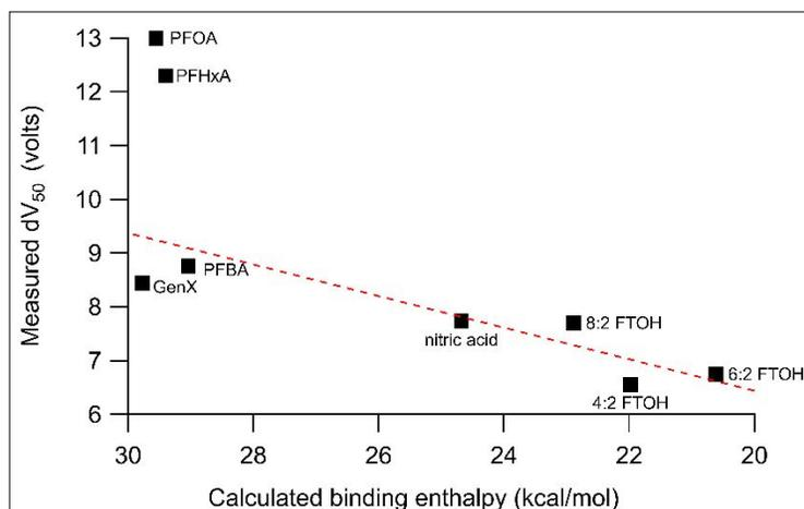
**Figure 5.** Relationship between calculated binding energy and measured  $dV_{50}$  for PFAS that formed clusters with iodide reagent ions and for nitric acid. The linear fit shown is just for nitric acid and the FTOHs, extrapolated to show that it's a poor fit for the PFCAs.
