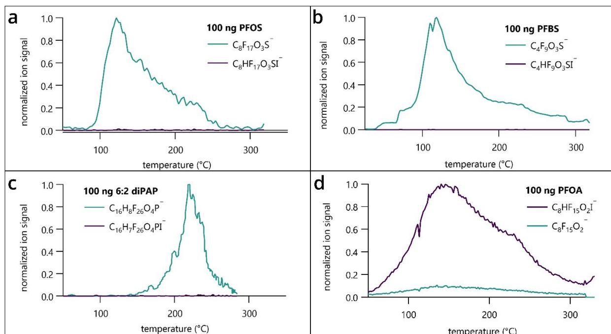
**Figure 6.** Normalized FIGAERO thermograms of aqueous solutions containing 100 ng of a) PFOS, b) PFBS, c) 6:2 diPAP, and d) PFOA. For all plots, the purple trace represents the iodide-PFAS cluster, while the teal trace represents a deprotonated PFAS anion.
