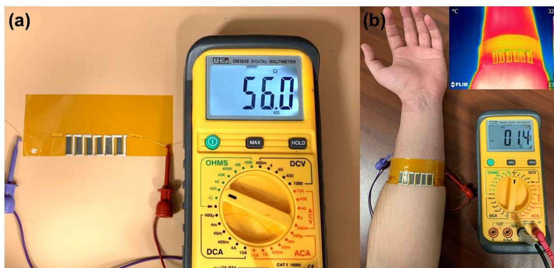
Figure 6. Performance of a wearable TEG. (a) Internal resistance of the TEG fabricated using six silver-selenide films. (b) The digital photo of 1.4 mV open-circuit voltage generated by \Delta T of \sim 1.8 \text{ K} between the hot-side and the cold-side of the device. The inset is the corresponding infrared thermal image.
