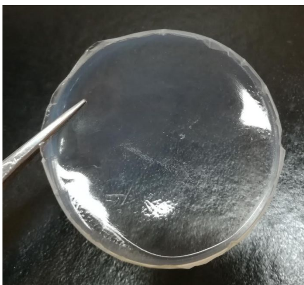
Figure 2: Image of the BMPyr-TFSI free standing film using 10 wt% PBDT and 90 wt% IL. Each film was controllably produced with a thickness of 100 – 200 \mu\text{m} , tailored to suit the needs of the characterization methods employed.
