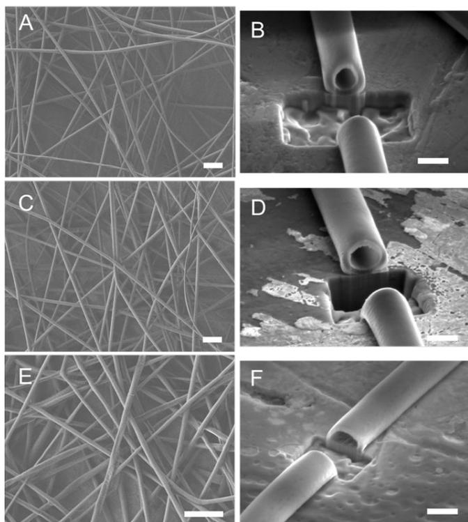
**Figure 4.** SEM images of nanofibers made with 0 wt% (A, B), 1.5 wt% (C, D), and 3 wt% (E, F) of  $C_4AzoC_6PEG_3$ . FIB-SEM images showing milled out sections of the fibers revealing the core-sheath morphology. Scale Bars: A, C, E = 10  $\mu\text{m}$ ; B, D, F = 1  $\mu\text{m}$ .
