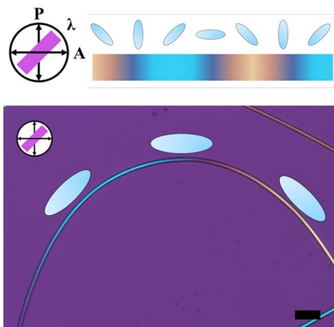
**Figure 6.** Electrospun nanofiber with 1.0 wt%  $C_4AzoC_6PEG_3$  and a 5CB core viewed with crossed POM and quarter-wave retardation plate showing axial planar alignment of the LC within the fiber. Color bar at top depicts how the image color corresponds to the LC orientation. Color change along the fiber indicates that the LCs are aligned along the fiber long axis. Scale bar = 10  $\mu m$ .
