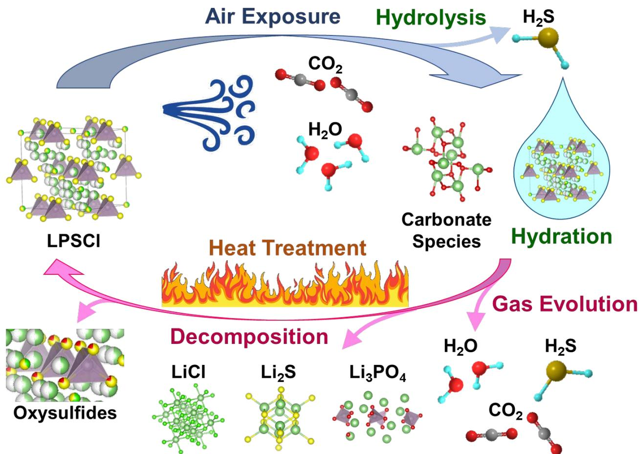
**Figure 1.** Schematic of the chemical reactions that occur when  $\text{Li}_6\text{PS}_5\text{Cl}$  is exposed to ambient air and during the subsequent heat treatment process.
