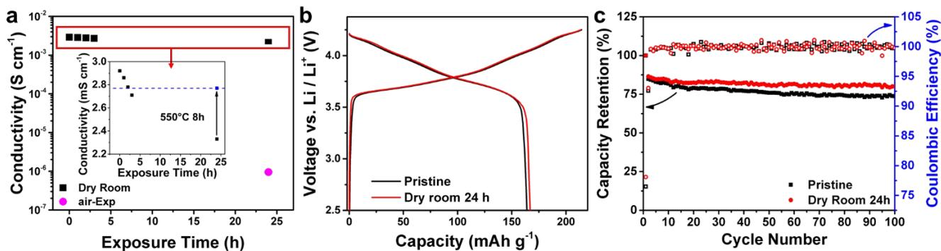
**Figure 6.** a) Ionic conductivity of pristine LPSCI, LPSCI samples exposed in a dry room for 1, 2, 3, 24 hours, a heat-treated sample following 24 hours of dry room exposure, and air-exposed LPSCI. b) 1<sup>st</sup> cycle voltage profiles, c) capacity retention and Coulombic efficiency of NCM811 | LPSCI | LiIn cells assembled using pristine or 24h dry room exposed LPSCI electrolytes.
