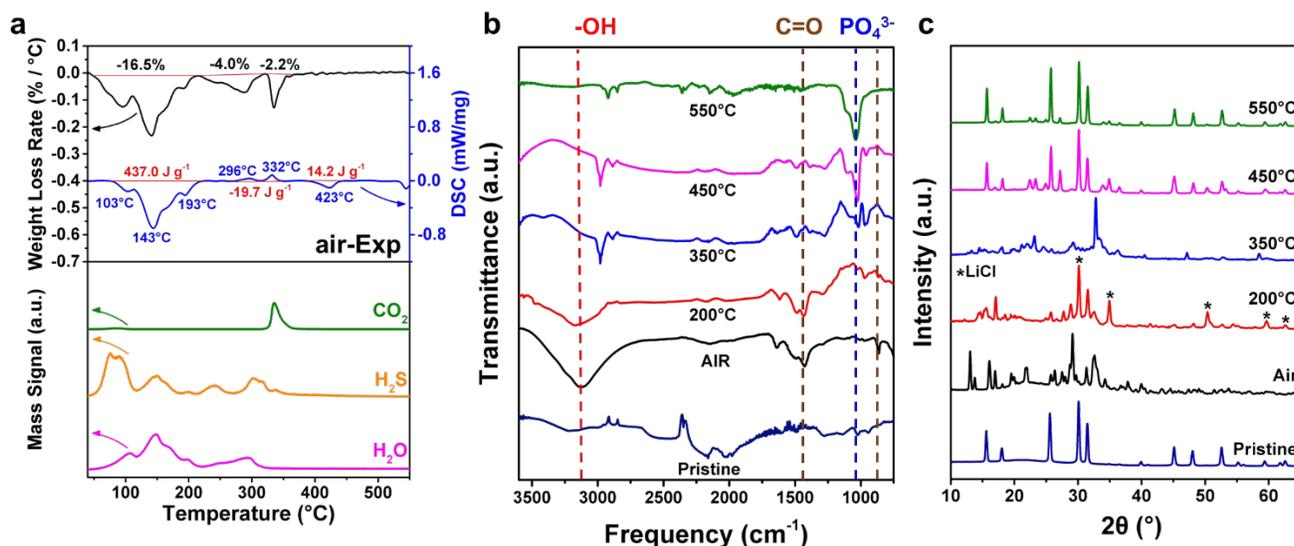
**Figure 5.** a) Coupled TGA / DSC and mass spectrometry measurements of the air exposed sample (air-Exp). b) FTIR spectra and c) XRD pattern of the air-Exp sample heat treated at different temperatures.
