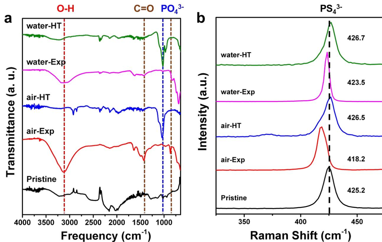
**Figure 3.** a) FTIR and b) Raman spectra of the pristine, exposed and heat-treated LPSi samples. The main peaks of interested are represented by dashed lines on the FTIR spectra, while the Raman spectra only shows the  $\text{PS}_4^{3-}$  peak.
