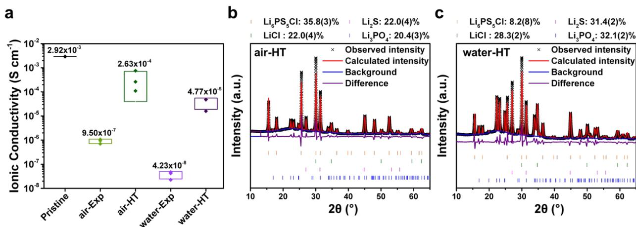
**Figure 2.** a) Ionic conductivity of the pristine, air, and water exposed LPSCl samples before and after heat treatment. All exposure and heat treatment conditions were conducted with three samples and median values are reported. Rietveld refinement results of the XRD patterns of b) the air exposed and heat-treated sample (air-HT) and c) the water exposed and heat-treated sample (water-HT). The molar phase ratios of all phases are labeled on top of the diffraction patterns.
