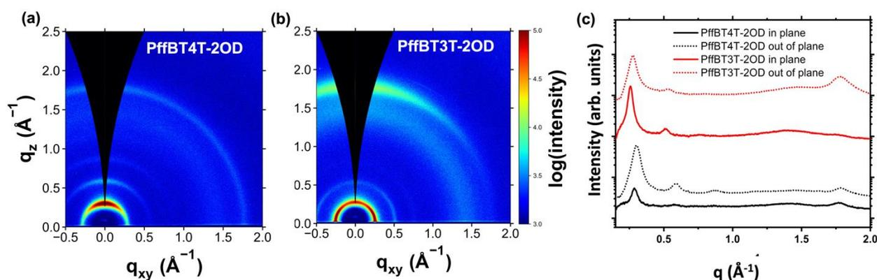
**Figure 5** 2D GIWAXS images of polymer thin films; (a) PffBT4T-2OD and (b) PffBT3T-2OD. (c) Integrated scattering intensity of GIWAXS measurements shown in (a) and (b).
