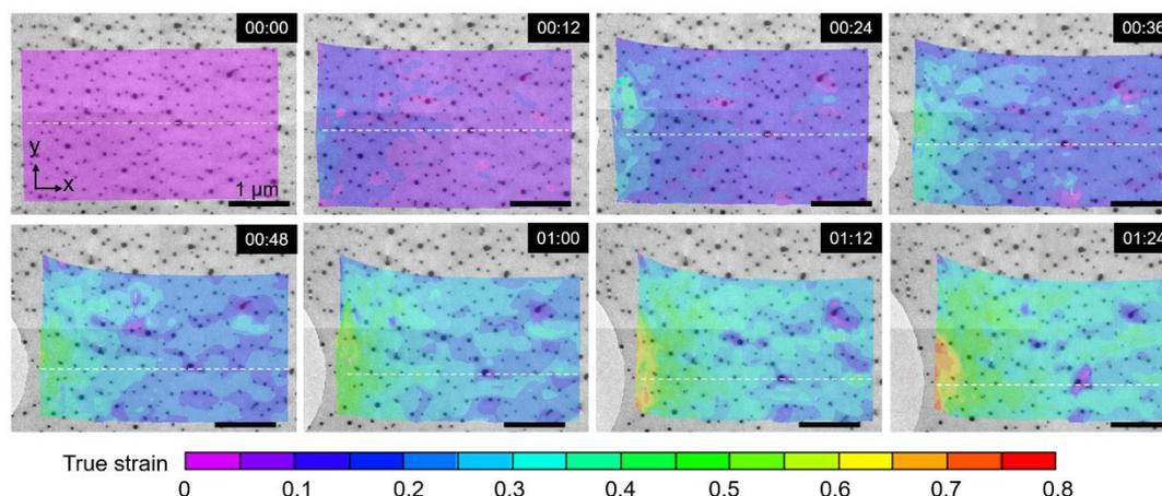
Figure 3. True strain distributions in the vicinity of the crack tip. The true strain in the upper-left figure is assumed to be zero. Tensile displacement was applied continuously at a rate of  $20 \text{ nm}\cdot\text{s}^{-1}$  in the  $y$  direction. The crack was expected to grow in the  $x$  direction. The true strain and strain rate along the white dashed line shown in each image are shown in Figure 4.
