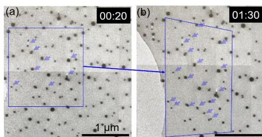
**Figure 2.** Nanovoids formed at the interfaces between silica nanoparticles and the epoxy matrix under different strain states. The region indicated by the blue rectangle in (a) (time = 00:20) changed into that in (b) (time = 01:30) as the tensile test proceeded. The formed nanovoids are indicated by light-blue arrows. Scale bars: 1  $\mu\text{m}$ .
