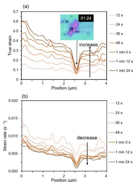
Figure 4. (a) True strain distributions along the  $y$ -axis under different tensile states (from 0 min, 12 s to 1 min, 24 s). Due to the presence of a large filler particle located approximately  $2,500 \text{ nm}$  from the crack tip, the generation of strain was constrained. (b) Calculated strain rates along the  $y$ -axis.
