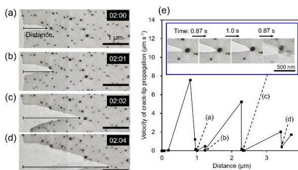
Figure 5. (a)–(d) TEM images of cracks propagating toward the right. The crack tips are arrested when they encounter silica nanoparticles. (e) The velocity of crack propagation as a function of the distance between the crack tip and the left edge of the film before crack formation. The insets in (e) show magnified TEM images of a crack suppressed by a silica nanoparticle. The time intervals between two sequential TEM images are also shown.
