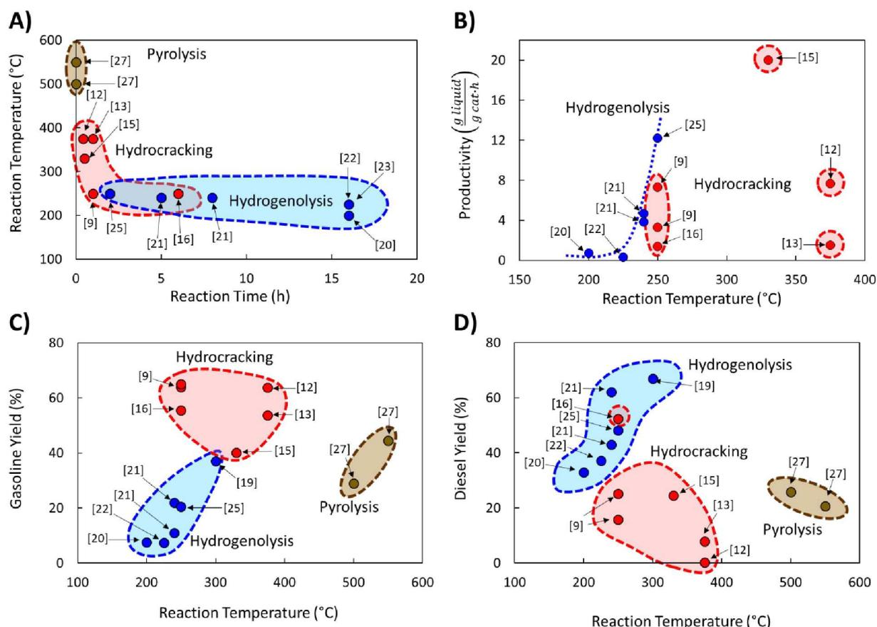
**Figure 1.** A) Correlation between reaction temperature and time for different PO upcycling strategies compared to pyrolysis for near complete conversion; B) Comparison of catalyst productivity to liquids with the remaining products being light gases and coke; C) Gasoline and D) diesel yields as function of reaction temperature. The brackets indicate the literature references. The colours distinguish the three processes.
