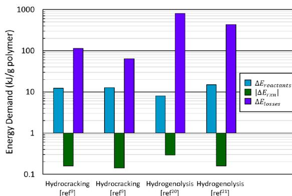
**Figure 3.** Relative contributions of energy terms for hydrocracking and hydrogenolysis in laboratory reactors. Blue: energy to bring reactants to reaction conditions; green: absolute value of reaction energy; and purple: energy lost to the surroundings for laboratory reactors (see text).
