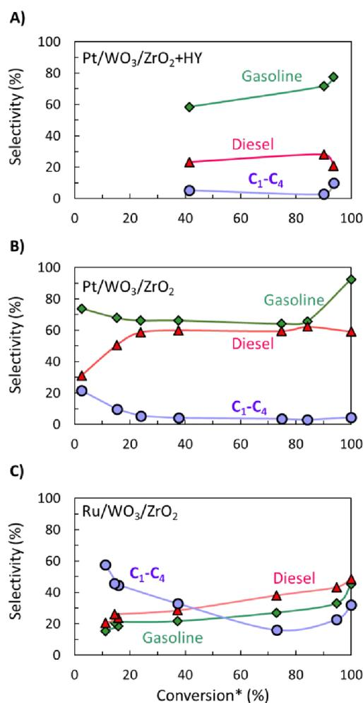
**Figure 2.** Selectivity to diesel, gasoline, and light gas hydrocarbons as function of apparent LDPE conversion for A) hydrocracking using a physical mixture of Pt/WO<sub>3</sub>/ZrO<sub>2</sub> and HY<sup>9</sup>; B) hydrogenolysis over a pure Pt/WO<sub>3</sub>/ZrO<sub>2</sub><sup>16</sup> and C) over Ru/WO<sub>3</sub>/ZrO<sub>2</sub><sup>25</sup>. \* - conversion was calculated based on total yield of liquid products.
