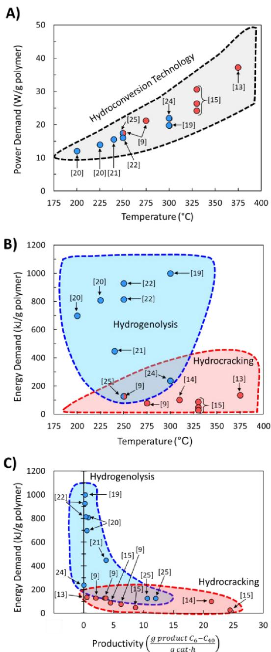
**Figure 4.** Correlations for laboratory reactors for A) power demand and reaction temperature; B) energy demand and temperature; and C) liquid productivity and energy demand for recent polyolefin hydroconversion literature.
