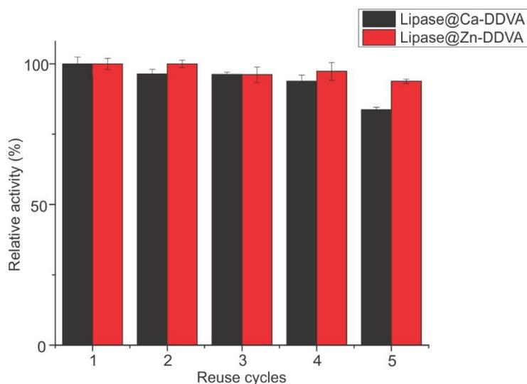
**Fig. 6. The relative reusability of the Ca-/Zn-DDVA MOF composites when lipase is studied as the model enzyme.** Within 5 cycles, both composites show  $\sim$ 80% relative catalytic efficiency. Lipase@Zn-DDVA shows higher reusability than lipase@Ca-DDVA.
