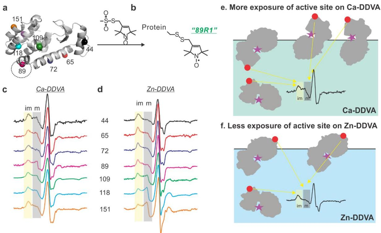
**Fig. 7. Probing the structural basis of the catalytic behavior using lys@MOM as a model system.** (a) The surface residues that are spin labeled with a nitroxide (b) for structural study. (c, d) The EPR spectrum of each labeled mutant upon encapsulation to each DDVA-based composites. (e, f) Schematic illustration of the exposable region of lys on Ca-DDVA and Zn-DDVA surface as determined via EPR. Star=lys active site.
