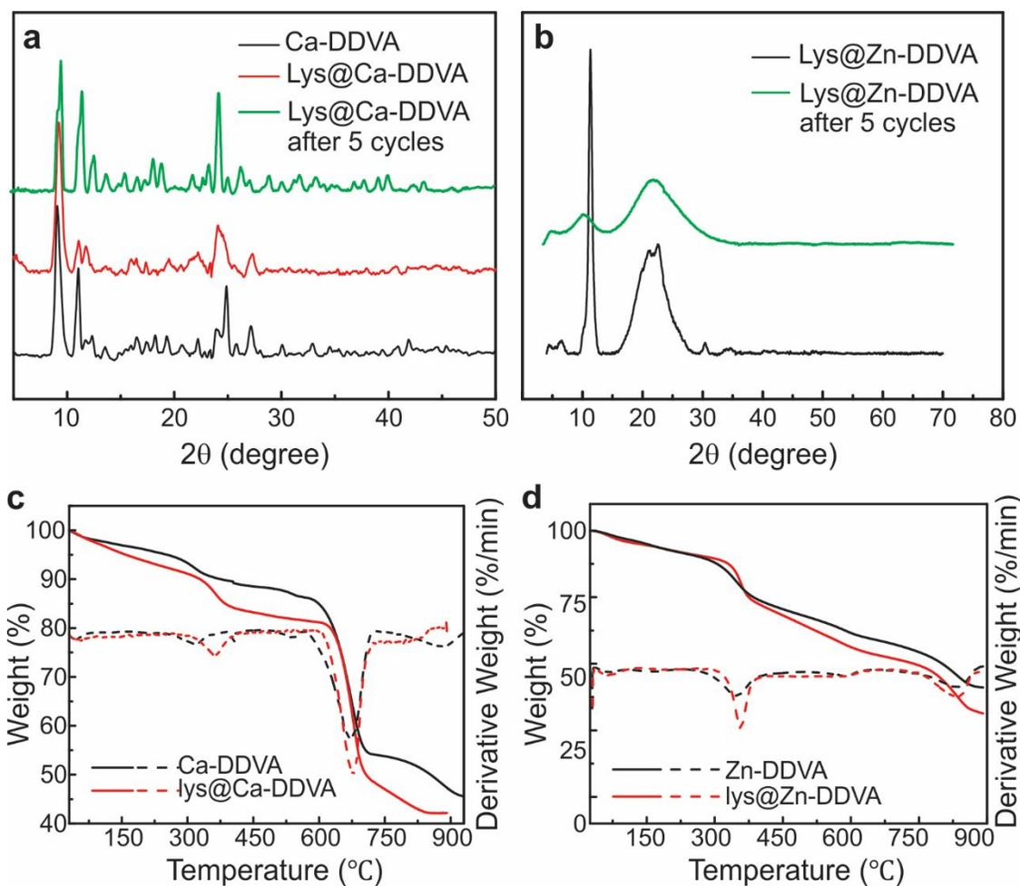
**Fig. 3. Characterization of the enzyme@Ca-/Zn-MOM composites.** (a) The XRD data of the lys@Ca-DDVA composites developed in this work before and after 5 catalytic cycles (green). (b) The PXRD of lys@Zn-DDVA before and after 5 catalytic cycles (green). (c) The TGA data of lys@Ca-DDVA as representatives of enzyme@MOM platforms suggested the inclusion of enzyme into the composites. (d) The TGA data of lys@Zn-DDVA.
