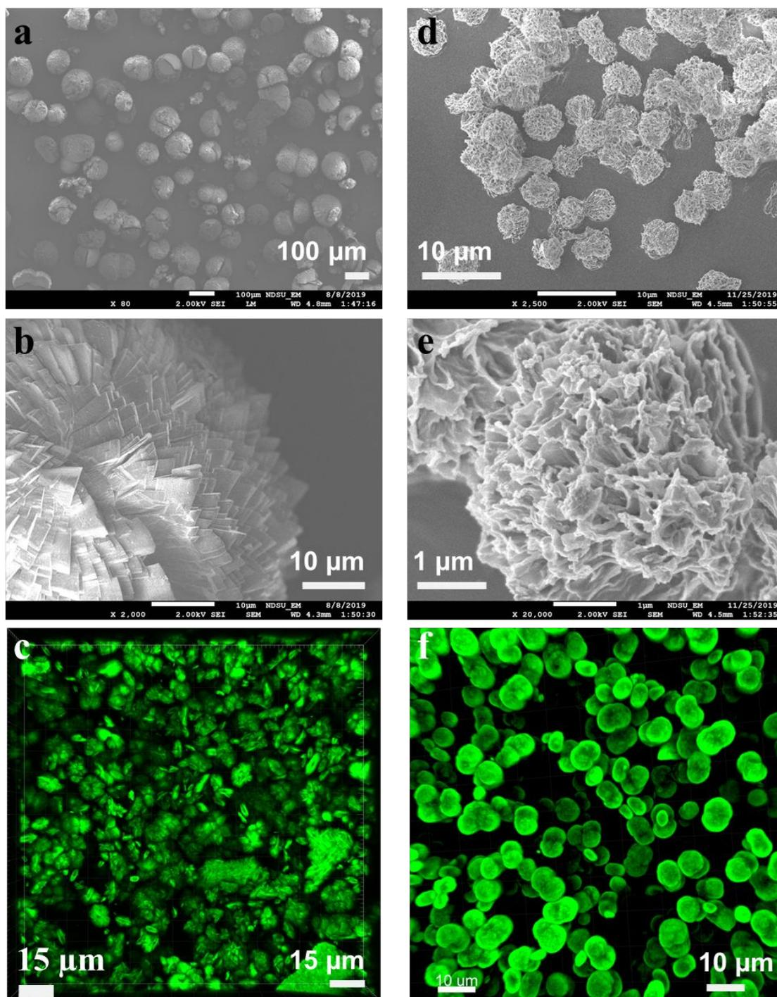
**Fig. 2.** Images of the enzyme@MOM composites. (a,b) The SEM images of the lys@Ca-DDVA at different length scales. (c) The confocal fluorescent images of FITC-labeled lys in Ca-DDVA. (d, e) The SEM images of the lys@Zn-DDVA at different length scales. (f) The confocal
