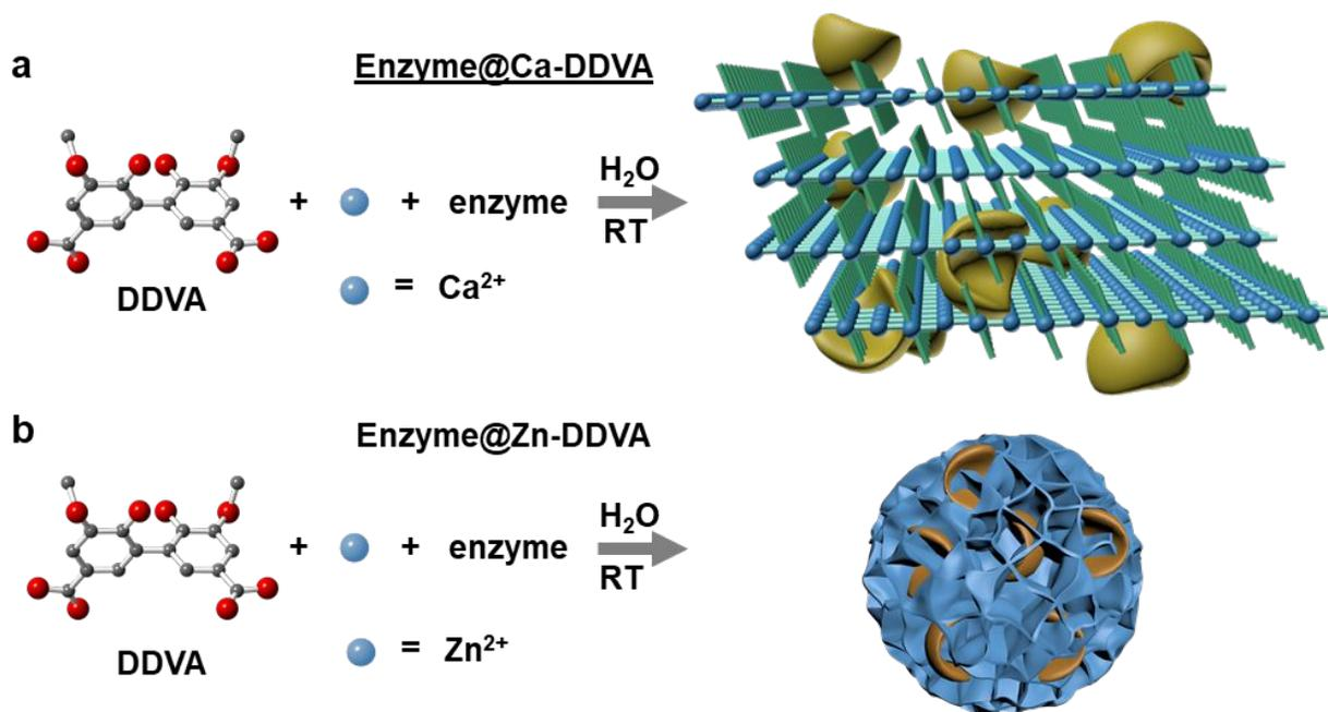
**Fig. 1. Reaction schemes of the preparation of the enzyme@Ca-MOM composites.** (a) Preparation of the enzyme@Ca-DDVA in water at room temperature (RT). (b) Preparation of the enzyme@Zn-DDVA in water at RT. The morphologies of the resultant composites are derived based on our experimental finding (see Fig. 2). Yellow/orange models represent enzymes in the composites.
