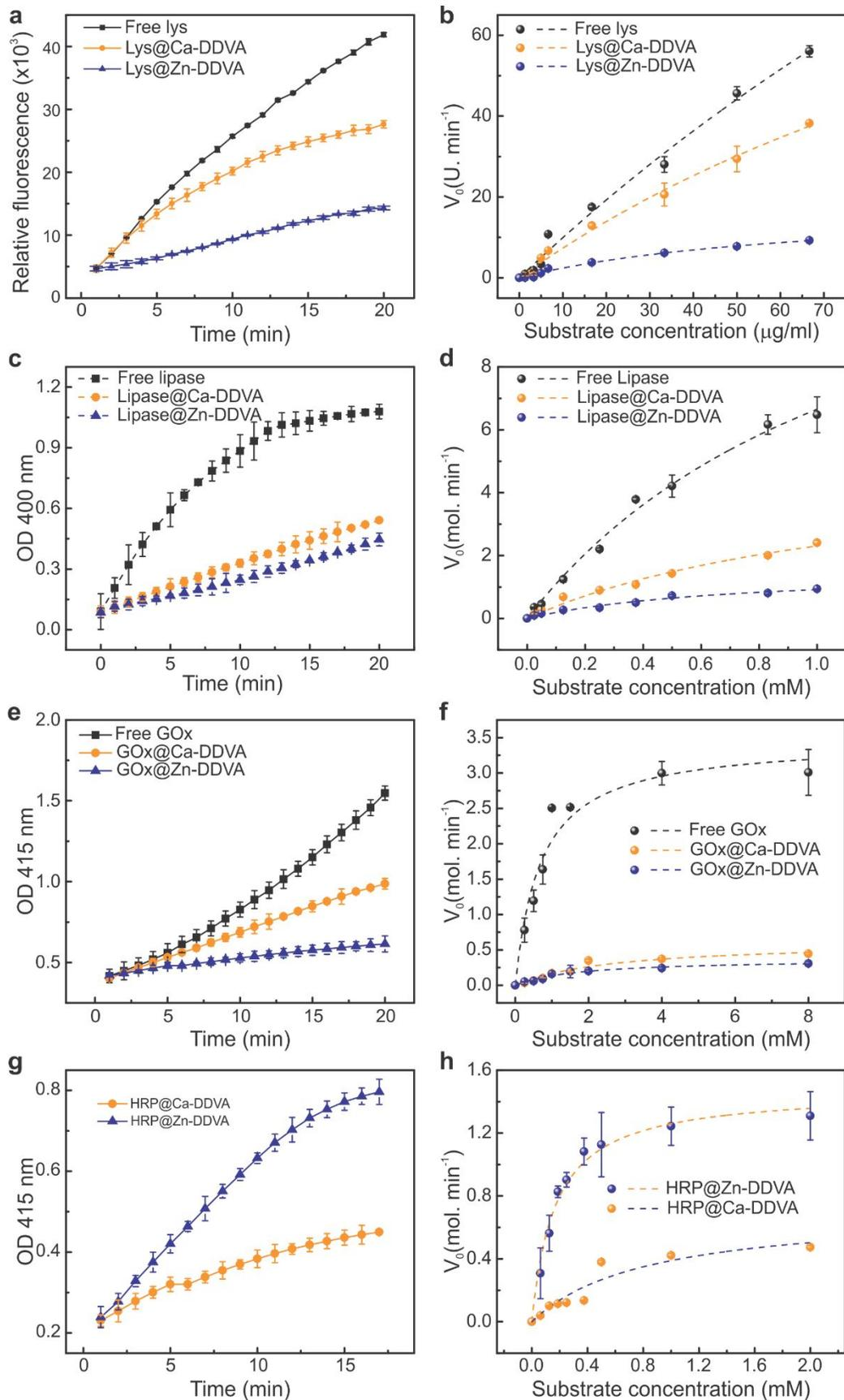
**Fig. 5. Activity assays of each enzyme@MOM composites.** (a,c,e,g) Representative data of the catalytic activity assays of lys (a), lipase (c), GOx (e), and HRP (g) upon loading into each composite. (b,d,f,h) The enzymatic kinetics analysis with fitting of each enzyme. Data analysis and fitting see the main text and the ESI.
