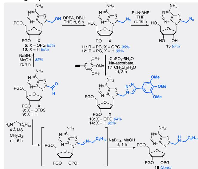
**Scheme 2** Transformations of silyl-protected 8-formyl derivatives of adenosine and 2'-deoxyadenosine (PG = *t*-BuMe<sub>2</sub>Si)
