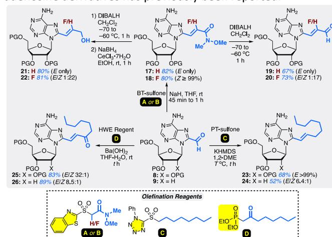
**Scheme 3** Olefination and fluoroolefination reactions of silyl-protected 8-formyl derivatives of adenosine and 2'-deoxyadenosine (PG = *t*-BuMe<sub>2</sub>Si)
