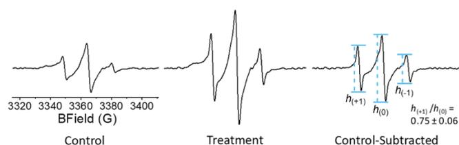
**Figure 4.** 100 G X-band EPR spectra of sialidase-treated HeLa cell after incubation with Neu5Ac9Az-CMP (without CSTII) and **2** (left, control), or with CSTII, Neu5Ac9Az-CMP and then **2** (middle), as well as cell count-normalized control-subtracted product spectrum (right).
