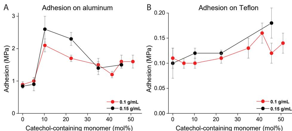
**Fig. 2** Adhesion for several variants of poly(catechol-MMA-OEG) on A) high energy aluminum substrates and B) low energy Teflon substrates.
