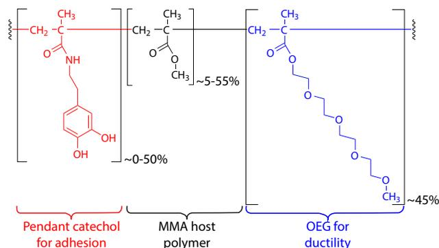
**Fig. 1** Poly(catechol-MMA-OEG) terpolymer used for structure-function studies on high energy aluminum and low energy Teflon. The OEG monomer content (blue) was held constant while the adhesive monomer (red) varied in loadings.
