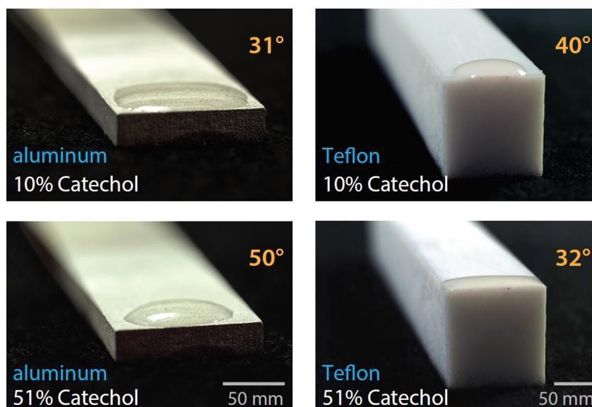
**Fig. 4** Wetting of aluminum (left) and Teflon (right) substrates by polymers in DCM/MeOH solutions with varying catechol content.
