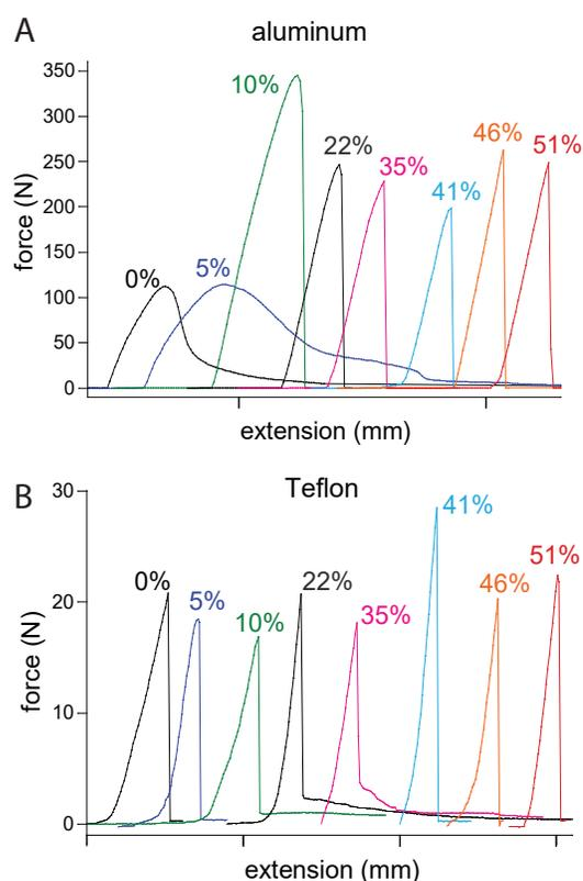
**Fig. 3** Force-versus-extension curves representative of several polymers on A) aluminum and B) Teflon. Each curve was offset on the x-axis for clarity. Note that the two plots are shown with different y-axis scales.
