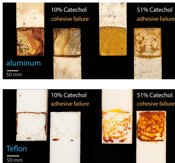
**Fig. 5** Variations in failure modes with poly(catechol-MMA-OEG) on aluminum (top) and Teflon (bottom). Higher bonding strengths occurred with more cohesive failure, which could be seen with 10 mol% catechol on aluminum and 51 mol% catechol on Teflon. Note that samples shown here were stained with iodine to aid visualizing the polymers. The same samples prior to staining can be seen in Fig. S7.
