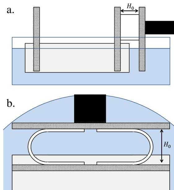
Fig. 2 A simplified adhesion measurement apparatus. a. shows a side view and b. shows a top down view. Light grey is the “boat”, black represents a rigid connection to the table, blue shows water in a crystallization bowl and glass plates are shown as cross-hatched rectangles. Two bent films are shown in white.
