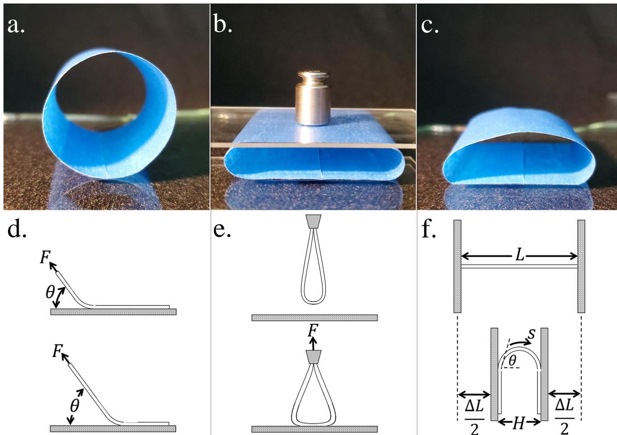
Fig. 1 Geometry of a tape loop. (a.) A tape loop resting on a clean glass surface. (b.) A compressed tape loop. (c.) A tape loop after compression is removed. (d.) schematic of a peel experiment. (e.) Schematic of a loop-tack test. (f.) Schematic of the tape loop experiment discussed here.
