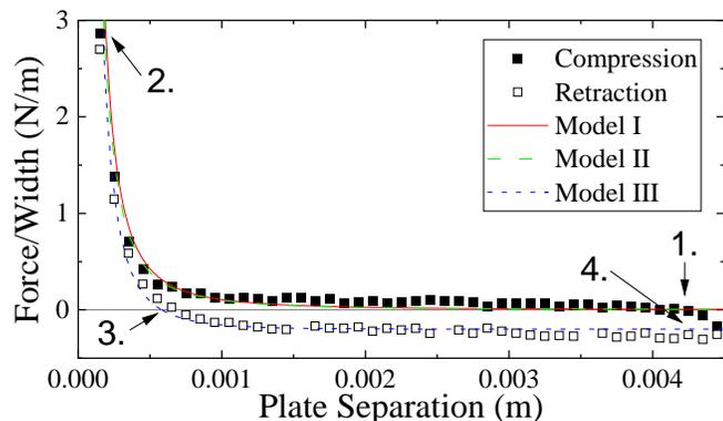
Fig. 3 A typical force displacement curve for a 10:1, thickness 56.4  $\mu\text{m}$  film. Fits to the circular, Rectangular Elastica and Sticky Elastica model are shown.
