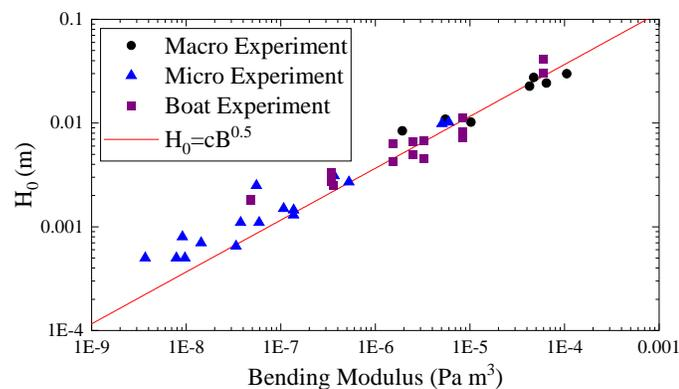
Fig. 7 Data validating the simple adhesion measurement.  $H_0$ , the plate separation at  $P = 0$ , is plotted against the bending modulus for various 10:1 PDMS films. Data from both macro and micro setups as well as the ‘boat’ experiments all fall along a common square-root curve as discussed in the text.
