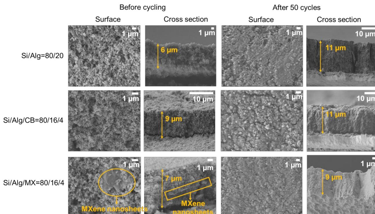
Figure 5: Scanning electron microscopy (SEM) images (both surface and cross section) of Si/Alg=80/20, Si/Alg/CB=80/16/4, and Si/Alg/MX=80/16/4 electrodes before and after 50 cycles.
