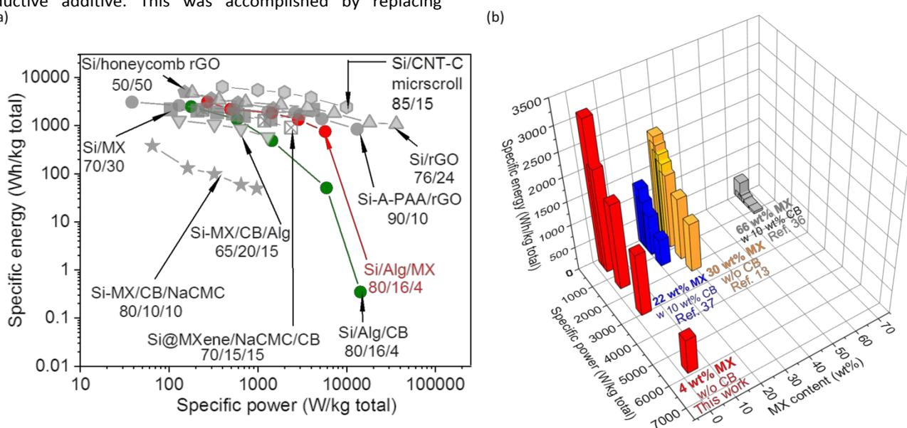
Figure 7: (a) Ragone plot of specific energy vs. specific power (W/kg). (b) 3D plot with specific energy, specific power (both based on total electrode mass), and MXene content (wt%). Table S3 summarizes the data displayed here.
