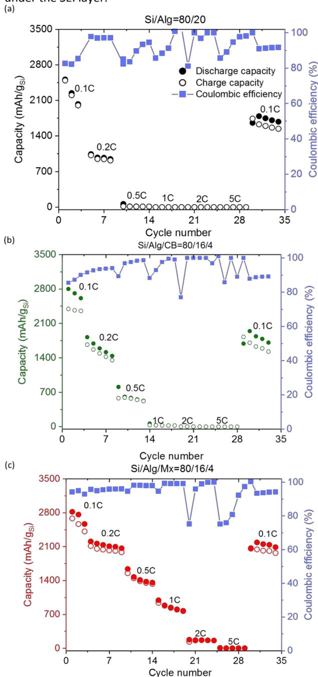
Figure 6: Rate performance at different C-rates ranging from 0.1 C to 5 C for (a) Si/Alg=80/20, (b) Si/Alg/CB=80/16/4, (c) Si/Alg/Mx=80/16/4 electrode. The active material loading was around  $0.70 \pm 0.05$  mg/cm<sup>2</sup>. The C-rate was brought back to 0.1 C again to determine the capacity recovery.
