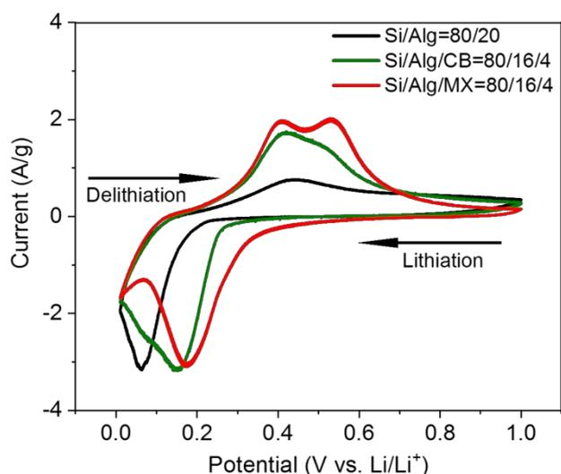
Figure 2: Cyclic voltammograms of Si/Alg=80/20, Si/Alg/CB=80/16/4, and Si/Alg/MX=80/16/4 at scan rate of 0.1 mV/s (third cycle is shown here). Cyclic voltammetry was performed for 5 cycles at 0.1 mV/s and the third cycle for each is shown here. The current is normalized by mass of silicon. Before CV, conditioning was performed at 0.1 C for 3 cycles.
