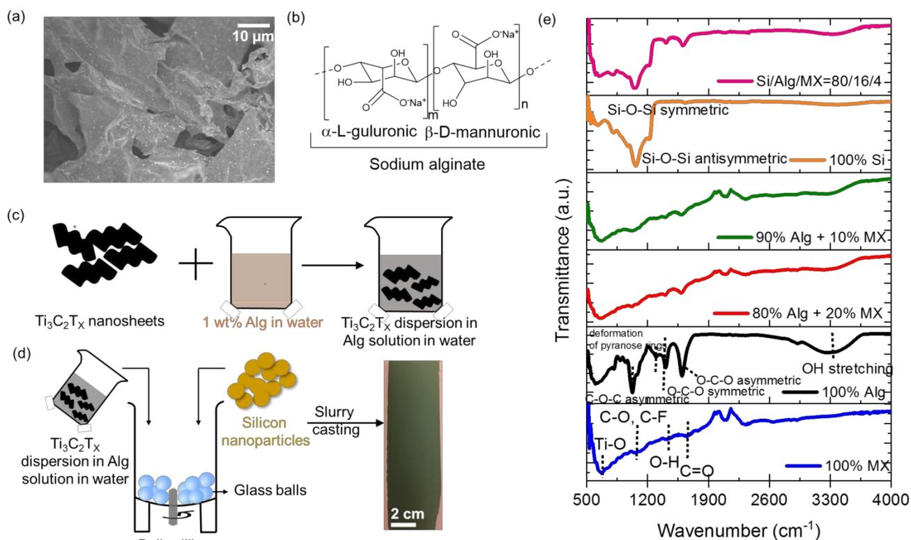
Figure 1: Scanning electron microscopy (SEM) image of  $\text{Ti}_3\text{C}_2\text{T}_x$  nanosheet, (b) schematic of sodium alginate (Alg), (c) schematic of a MXene dispersion in aqueous Alg solution, (d) schematic of electrode fabrication process by simple slurry casting method, and (e) FTIR spectra of MXenes, Alg, 90 wt% Alg + 10 wt% MX, 80 wt% Alg + 20 wt% MX.
