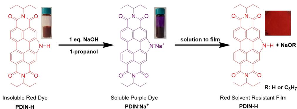
**Figure 1.** Chemical structure of PDIN-H. Treatment of a 10 mg/mL slurry of PDIN-H in 1-propanol with 1 molar equivalent of NaOH produces a purple ionic solution. Spin-coating this solution onto a PET substrate yields a red colored organic film owing to the spontaneous protonation of the PDIN anion. This process mimics that of classic acid dyeing of textiles.
