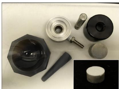
Fig. 1 Pellet sample creation equipment used in this study, with inset example of final pellet form. Photo was taken from Wood 2020.<sup>43</sup>
